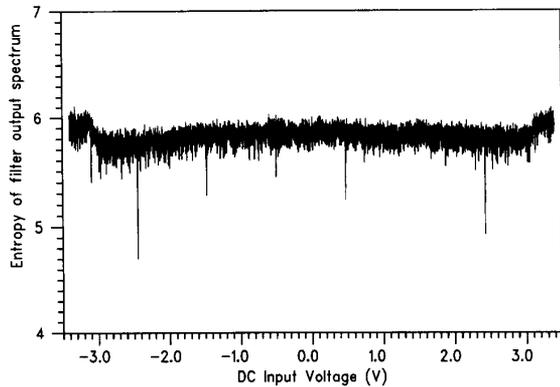
Fig. 14. Spectral entropy versus dc input voltage.
