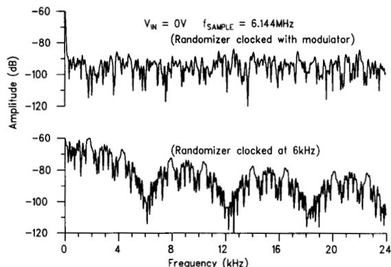
Fig. 7. Measured noise during calibration.
