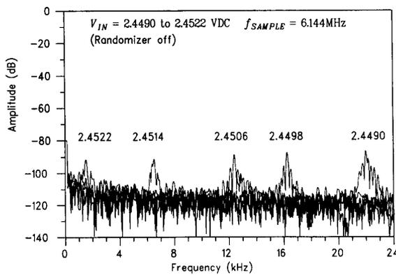
Fig. 15. Tone energy at various dc input voltages.
