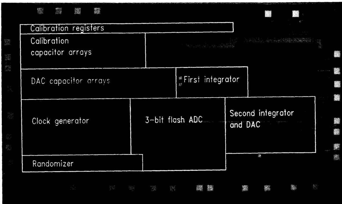
Fig. 19. Chip photomicrograph.
