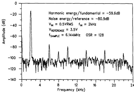
Fig. 9. Uncalibrated DAC and randomizer off.
