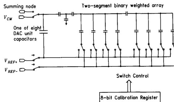
Fig. 3. Capacitor calibration networks.
