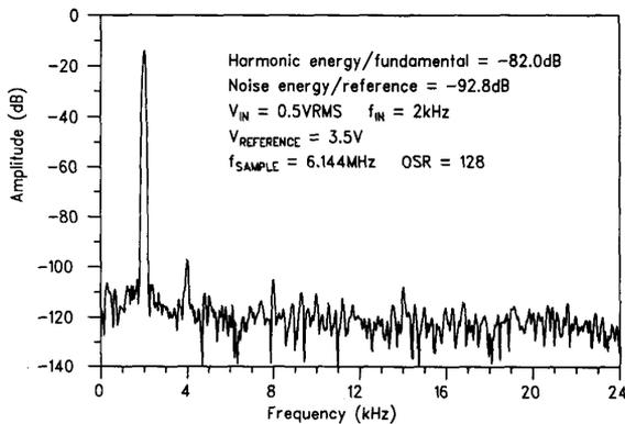
Fig. 11. Calibrated DAC and randomizer off.
