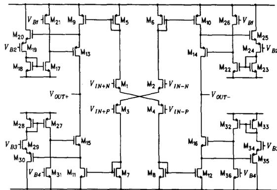
Fig. 5. Class AB op amp for first integrator.
