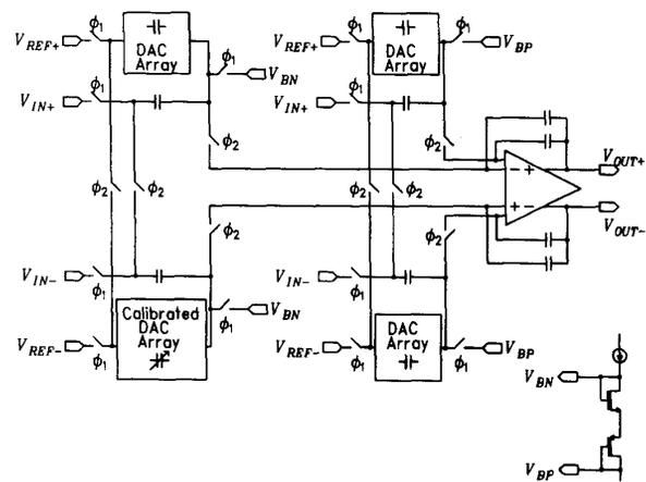
Fig. 6. First integrator schematic.
