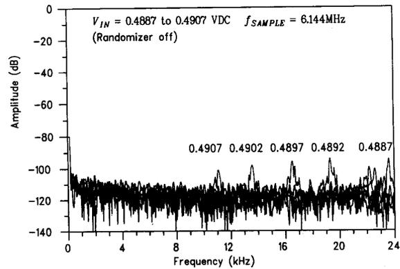
Fig. 17. Tone energy at various dc input voltages.
