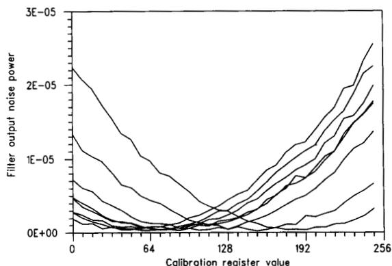
Fig. 8. Calibration noise versus calibration register value.
