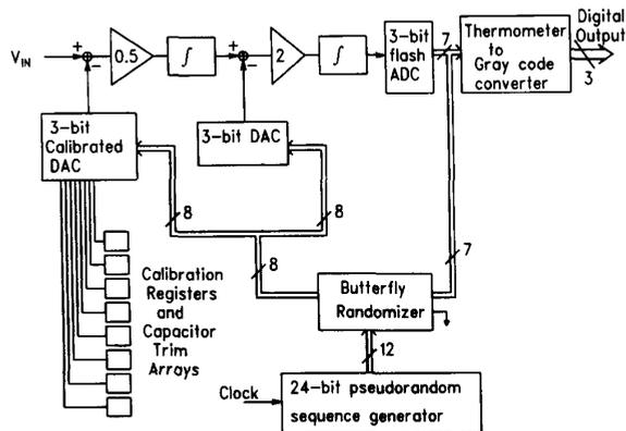
Fig. 1. Modulator block diagram.
