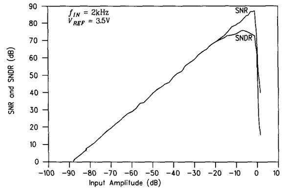
Fig. 13. SNR and SNDR versus input amplitude.
