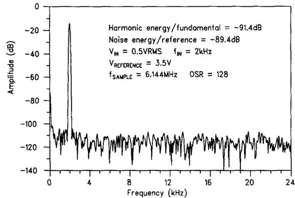
Fig. 12. Calibrated DAC and randomizer on.
