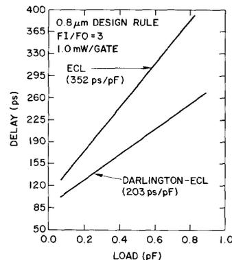
Fig. 6. Delays versus capacitive loading for the conventional ECL and the Darlington ECL circuit ( $0.8\text{-}\mu\text{m}$  design rule,  $FI/FO = 3, 1\text{ mW/gate}$ ).
