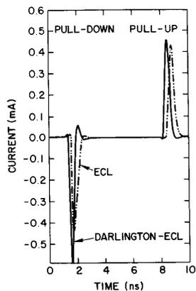
Fig. 2. Net pull-up and pull-down currents during the switching transient for the conventional ECL circuit and the Darlingtion ECL circuit (0.8- $\mu\text{m}$  design rule,  $FI/FO = 3$ ,  $C_L = 0.3$  pF, 1 mW/gate).
