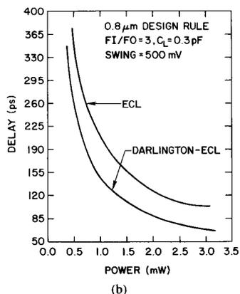
Fig. 4. (a) Unloaded ( $FI/FO = 1$ ) power-delay characteristics, and (b) loaded ( $FI/FO = 3$ ,  $C_L = 0.3$  pF) power-delay characteristics for the conventional ECL circuit and the Darlingtion ECL circuit at 0.8- $\mu\text{m}$  design rule.
