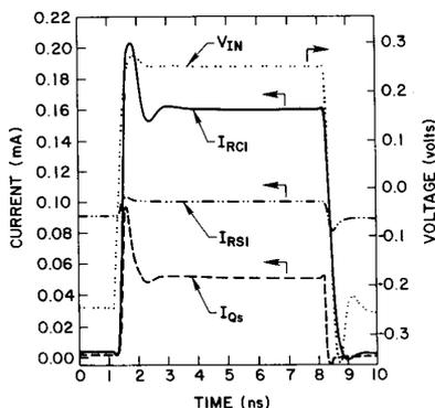
Fig. 3. Pertinent waveforms during the switching transient for the Darlingtion ECL circuit.  $V_{IN}$  is the voltage at the input,  $I_{RS1}$  is the current flowing through the (current source) resistor  $R_{S1}$ ,  $I_{Qs}$  is the current flowing through the dynamic current source transistor  $Q_S$ , and  $I_{RC1}$  is the current flowing through the load resistor  $R_{C1}$  (0.8- $\mu\text{m}$  design rule,  $FI/FO = 3$ ,  $C_L = 0.3$  pF, 1 mW/gate).
