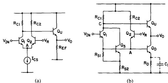
Fig. 1. Schematics of (a) conventional ECL circuit (the current source  $I_{CS}$  can be implemented either by a resistor or by a transistor current source), and (b) Darlington ECL circuit.
