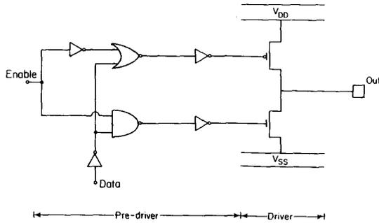
Fig. 7. High-speed, tri-statable (enable low) CMOS output driver.
