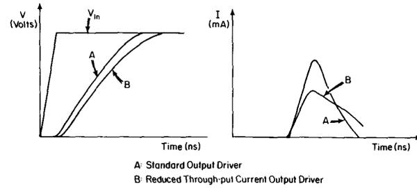
Fig. 8. Tri-State output driver switching characteristics.
