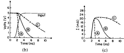
Fig. 3. (a) CMOS output driver switching characteristics. (b) Voltage switching characteristics. (c) Current switching characteristics. Here  $C_{Load}$  for case A = 0 pF, B = 26 pF, and C = 100 pF.
