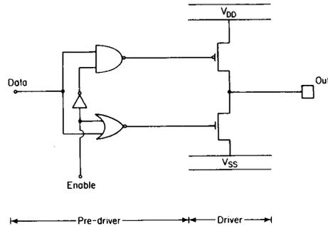
Fig. 6. A typical tri-statable (enable high) CMOS output driver.
