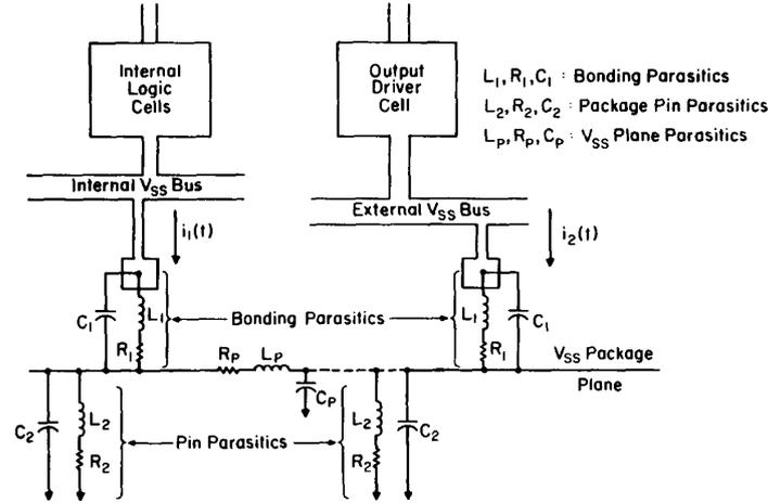
Fig. 1. A typical chip-package interface [2].
