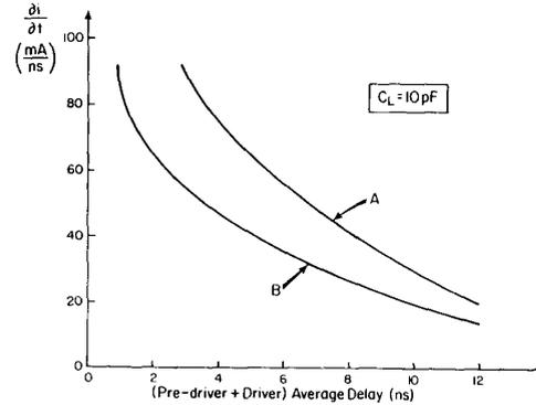
Fig. 9. Driver delay-switching noise limitations.
