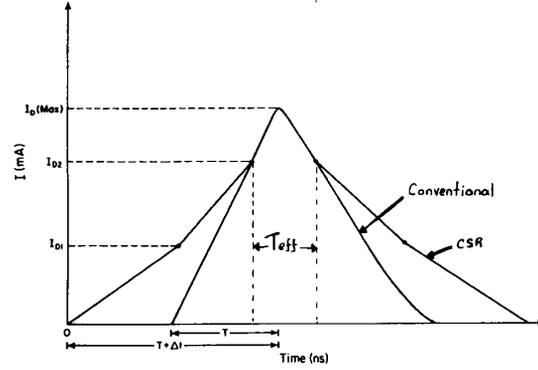
Fig. 12. CSR output driver current switching characteristics.
