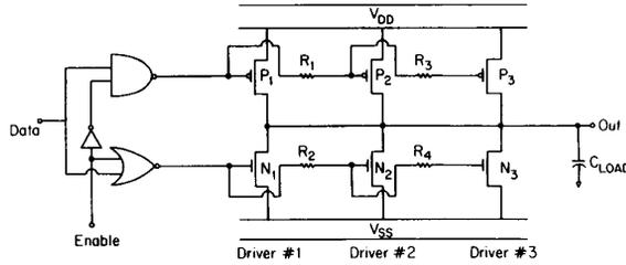
Fig. 10. Tri-statable, Controlled Slew Rate (CSR) output driver.
