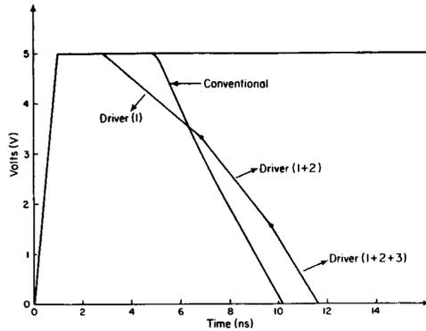
Fig. 11. CSR output driver voltage switching characteristics.
