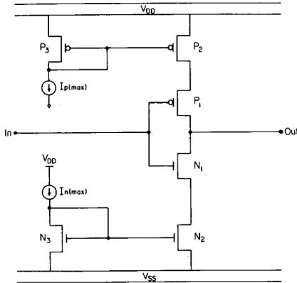
Fig. 4. Current controlled CMOS output driver.
