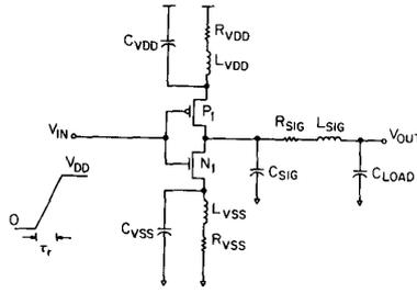
Fig. 2. Output driver final stage equivalent circuit [2].
