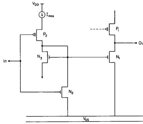
Fig. 5. Switching current controlled/unregulated CMOS output driver.
