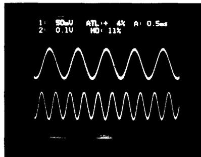
Fig. 15. Input and output waveforms of the basic squaring circuit. (Upper: input waveform, Lower: output waveform).
