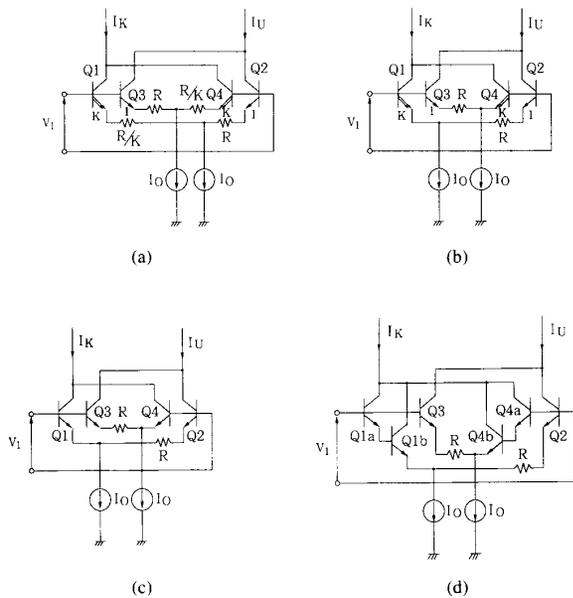
Fig. 10. Squaring circuits consisting of unbalanced emitter-coupled pairs with unbalanced emitter degeneration. (a) Transistor-pair with emitter area ratio  $K$  and degeneration resistor ratio  $1/K$ . (b) Transistor-pair with emitter area ratio  $K$  and an emitter resistor. (c) Transistor-pair with one side emitter resistor. (d) Transistor-pair of a Darlington-pair and a transistor with an emitter resistor.
