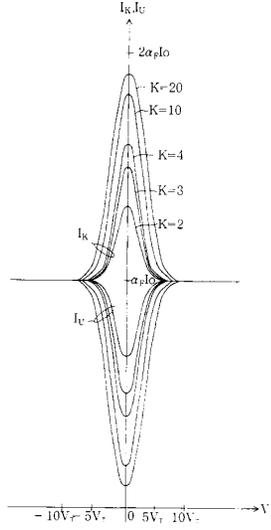
Fig. 2. DC transfer curves of a basic squaring circuit consisted of two identical unbalanced emitter-coupled pairs with emitter area ratio  $K$ .
