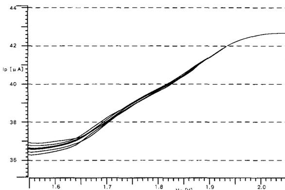
Fig. 14. Device mismatch effects on the quarter-square multiplier simulated with SPICE.
