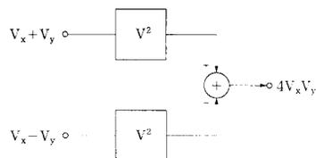
Fig. 5. A quarter-square multiplier block diagram showing cross-coupled outputs of two identical squaring circuits.
