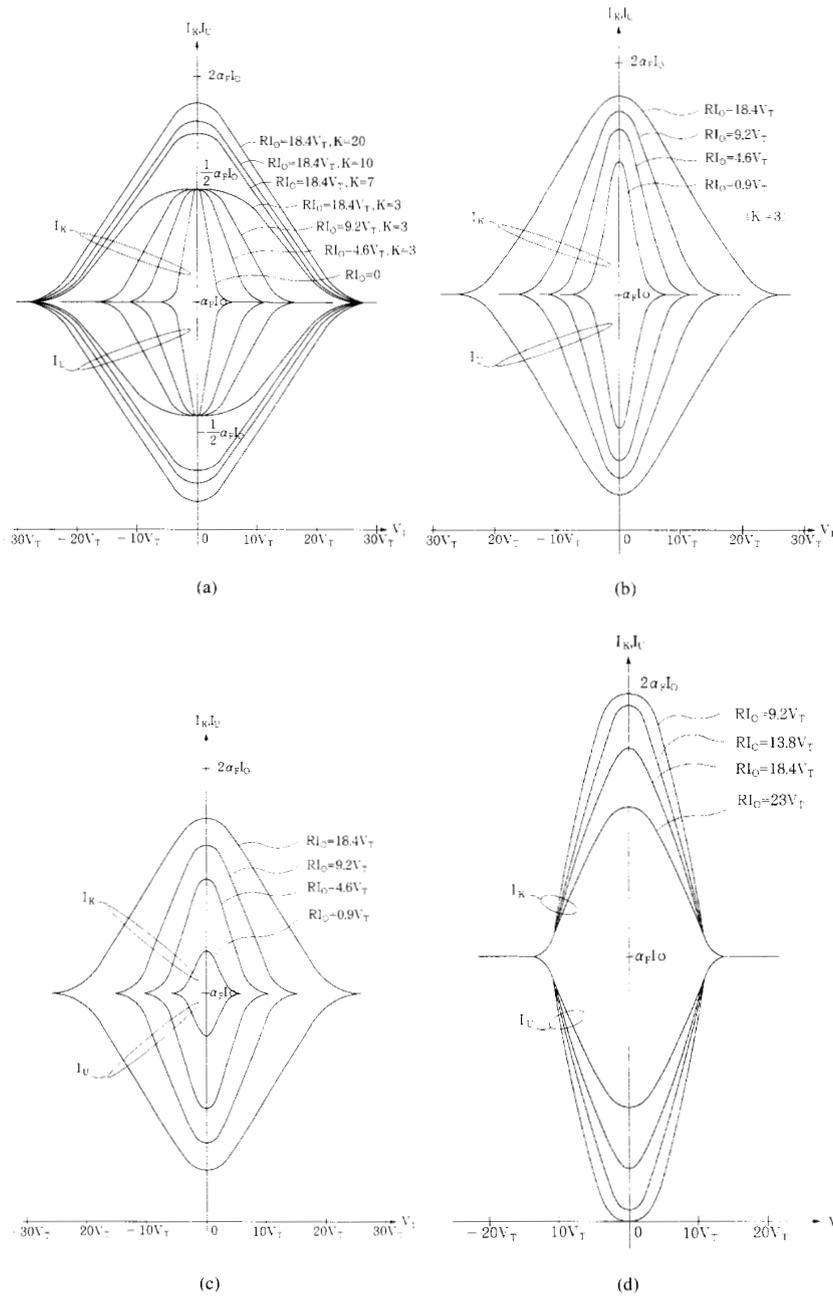
Fig. 11. SPICE simulations of the squaring circuits consisted of unbalanced emitter-coupled pairs for various values of  $R_{I0}$ . (a) Transistor-pair with emitter area ratio  $K = 3$  and the degeneration resistor ratio  $1/K = 1/3$ . (b) Transistor-pair with emitter area ratio  $K = 3$  and an emitter resistor. (c) Transistor-pair with one side emitter resistor. (d) Transistor-pair of a Darlington-pair and a transistor with an emitter resistor.
