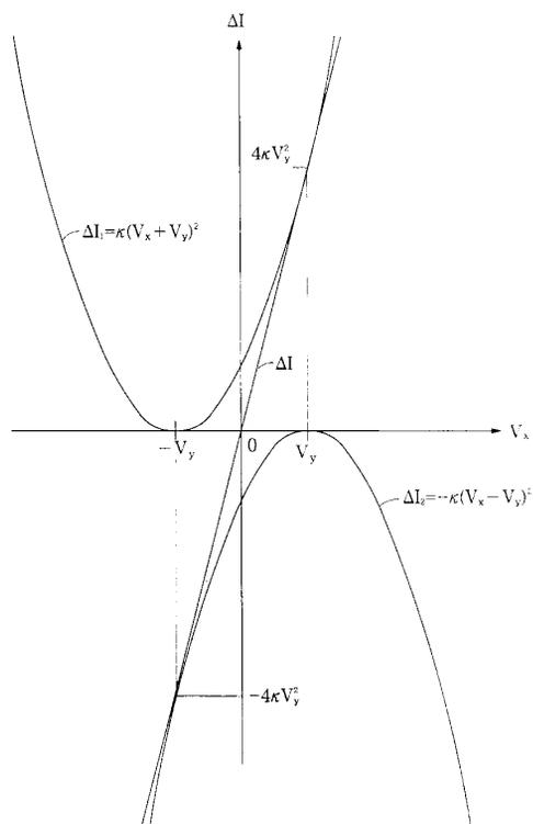
Fig. 6. A graphical illustration of linear behavior for a four-quadrant analog multiplier based on the quarter-square technique.
