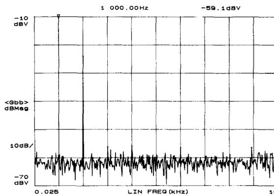
Fig. 16. Output spectrum of the basic squaring circuit.
