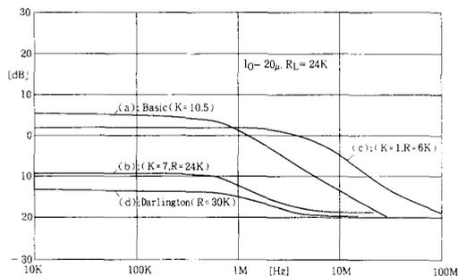
Fig. 13. Frequency characteristics of the quarter-square multipliers simulated with SPICE.
