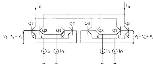
Fig. 7. A basic quarter-square multiplier consisted of four identical unbalanced emitter-coupled pairs with emitter area ratio  $K$ .
