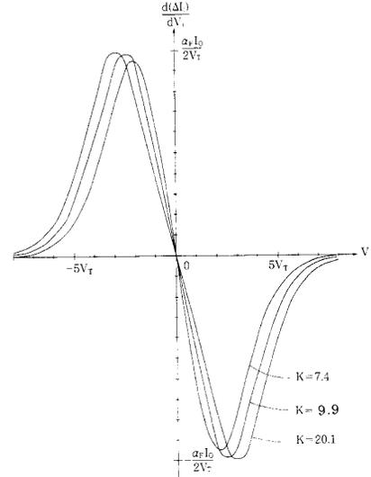
Fig. 3. Transconductance of a basic squaring circuit consisted of two identical unbalanced emitter-coupled pairs with emitter area ratio  $K$ .
