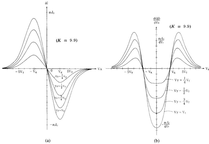
Fig. 8. DC characteristics of a basic quarter-square multiplier. (a) Transfer curves for four values of  $V_y$ . (b) Transconductance characteristics for four values of  $V_y$ .
