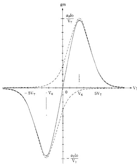
Fig. 9. Short-circuit transconductance of a basic quarter-square multiplier.
