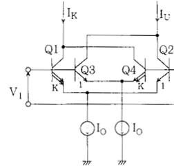
Fig. 1. A basic squaring circuit consisted of two identical unbalanced emitter-coupled pairs with emitter area ratio  $K$ .
