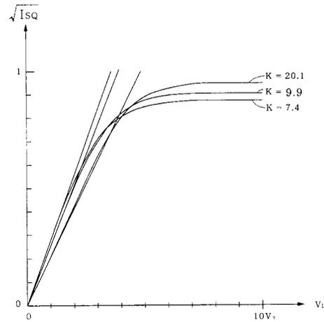
Fig. 4. Relationship between the square-root of the differential output current of a basic squaring circuit consisted of two identical unbalanced emitter-coupled pairs with emitter area ratio  $K$  and the differential input voltage  $V_1$ .
