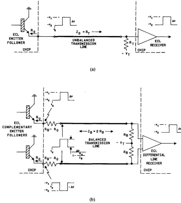
Fig. 2. The unbalanced and balanced ECL driver circuits dissipate equal average power when  $R_B = R_T + R_0/2$ . (a) Unbalanced driver circuit, impedance matched at one end. (b) Balanced driver circuit, impedance matched at both ends.
