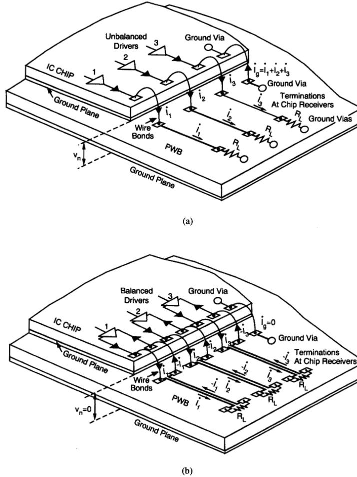
Fig. 1. AC circuits for unbalanced and balanced drivers. (a) AC circuit for unbalanced drivers. (b) AC circuit for balanced drivers.
