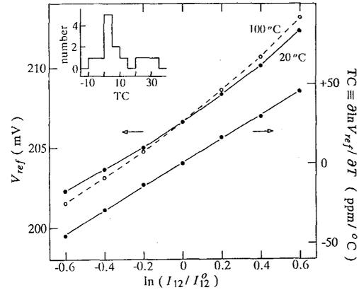
Fig. 3. Temperature and bias dependence of new feedback circuit prototype using CA3046 transistor array. Component values were  $R_1 = 383$   $\Omega$ ,  $R_2 = 2.37$  k $\Omega$ ,  $R_3 = 3.83$  k $\Omega$ ,  $K = 27$ . Zero TC point occurs at  $I_{12}^0 = 1$  mA.
