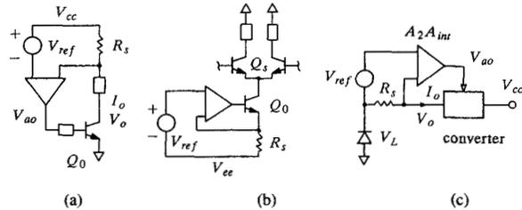
Fig. 1. Three common circuits where the operating point is established by current regulation: (a) linear or limiting amplifier, (b) laser or line driver, (c) LED or high power laser bias circuit.
