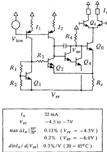
Fig. 5. Line driver bias circuit using new topology. This circuit demonstrates that intermediate amplifier does not compromise simplicity.
