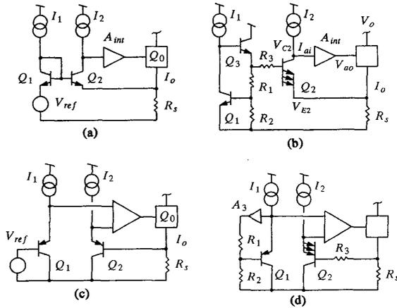
Fig. 2. Conventional current sensing feedback topologies using separate reference and error amplifier (a), (c). Proposed improved feedback amplifier topologies incorporating an internal low voltage bandgap reference (b), (d).  $A_{int}$  denotes the intermediate amplifier.
