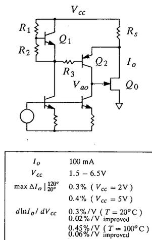
Fig. 4. MESFET amplifier bias circuit using CA3096CE transistor array.  $m \approx 10$  is achieved using just two transistors in the array by substituting an npn in place of a pnp device for  $Q_1$ .
