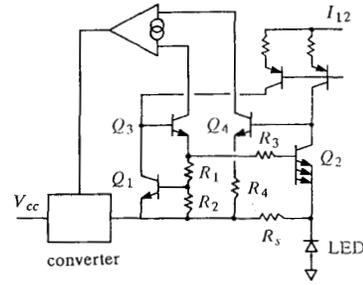
Fig. 6. Feedback circuit for biasing LED which further improves common mode rejection.
