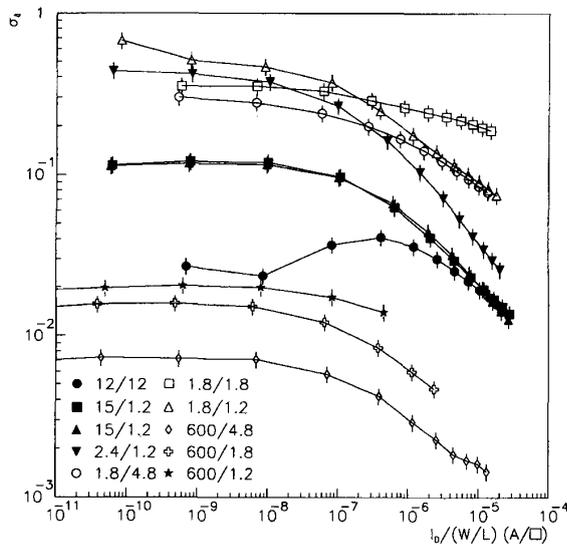
Fig. 2. Current mismatch versus current density for Mosis/HP 1.2- $\mu\text{m}$  NMOS transistors. Note the crossing lines of the small transistors with small W/L ratio. The PMOS transistors show a similar behavior.
