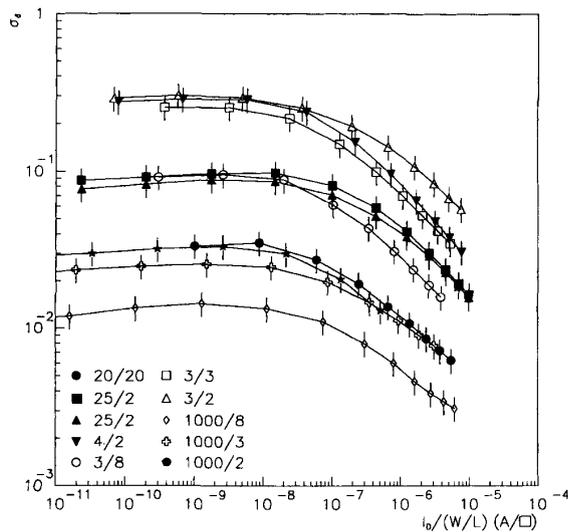
Fig. 3. Current mismatch versus current density for Mosis/Orbit 2- $\mu\text{m}$  NMOS. The PMOS transistors show a similar behavior.
