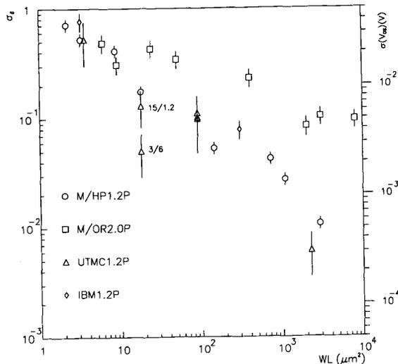
Fig. 5. Current and voltage mismatch versus drawn device area for all processes, PMOS transistors at  $I_{\square} = 1 \text{ nA}/\square$ .
