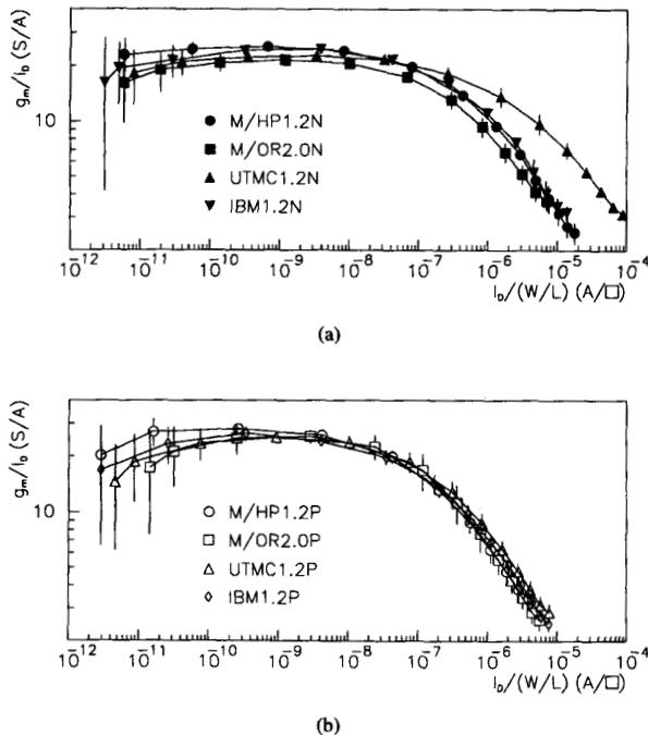
Fig. 1. Average  $g_m/I_D$  versus  $I_D$  for all transistor sizes and all processes. The error bars represent the spread of  $g_m/I_D$ .
