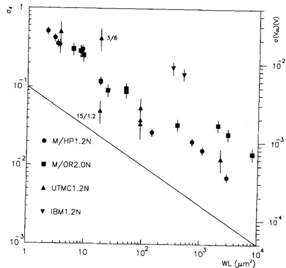
Fig. 4. Current and voltage mismatch versus drawn device area for all processes NMOS transistors at  $I_{\square} = 1 \text{ nA}/\square$ . The straight line represents the slope of the expected  $1/\sqrt{WL}$  dependence.
