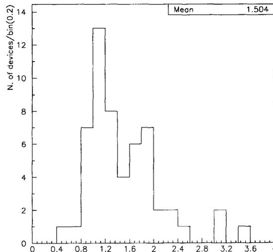
Fig. 6. Distribution of the ratio  $\sigma_{\delta}(V_{SUB} = 1) / \sigma_{\delta}(V_{SUB} = 0)$  for all device at  $I_{\square} = 1 \text{ nA}/\square$ .
