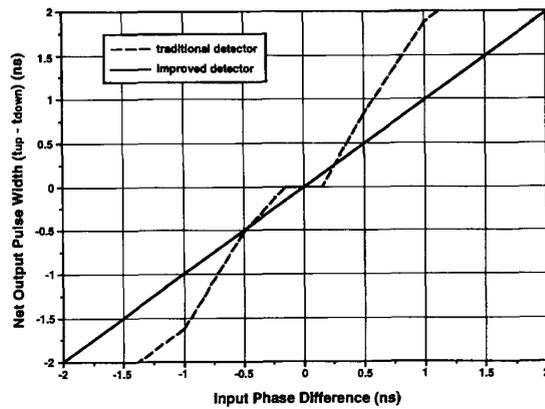
Fig. 4. Phase frequency detector transfer characteristic.
