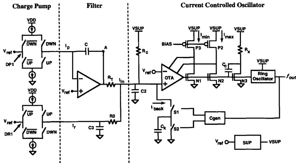
Fig. 5. PLL charge pump, loop filter, and current-controlled oscillator.
