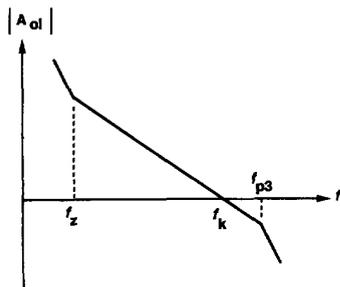
Fig. 6. Bode plot of PLL open-loop gain.
