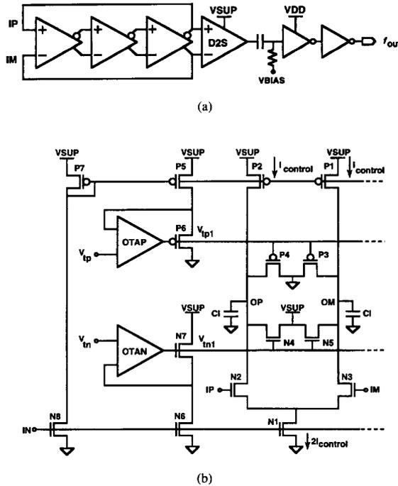
Fig. 7. (a) Ring oscillator. (b) Ring oscillator detail.
