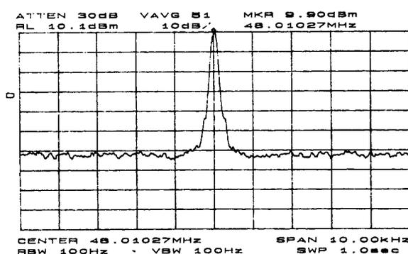
Fig. 12. Spectral analysis of synthesized frequency.
