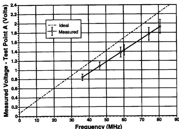
Fig. 11. VCO transfer characteristic: measured versus ideal.
