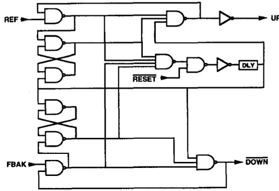
Fig. 3. Phase frequency detector block diagram.
