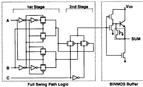
Fig. 5. Adder circuit for multiplier.
