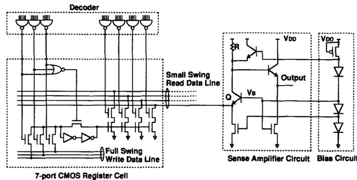
Fig. 3. Register file with single-ended common-base sense circuit.
