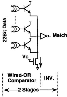
Fig. 4. Twenty-two bit comparator circuits for TLB.
