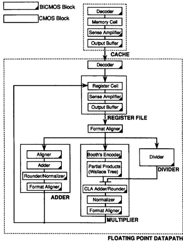
Fig. 2. Floating point datapath and cache block diagram.
