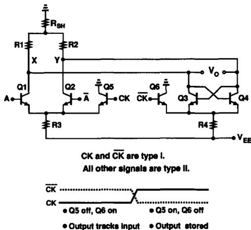
Fig. 4. D-latch circuit diagram.
