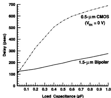
Fig. 14. Delay of bipolar and CMOS line drivers versus load capacitance.
