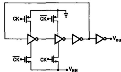
Fig. 11. CMOS frequency divider.
