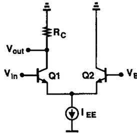
Fig. 19. Single-ended bipolar differential pair.
