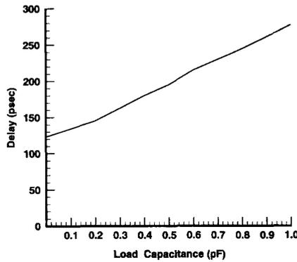
Fig. 9. Simulated delay of buffer/level shifter versus load capacitance.
