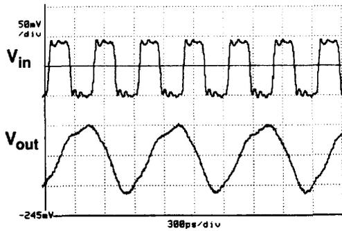
Fig. 17. Measured bipolar divider waveforms at  $f_{in} = 2.2$  GHz.
