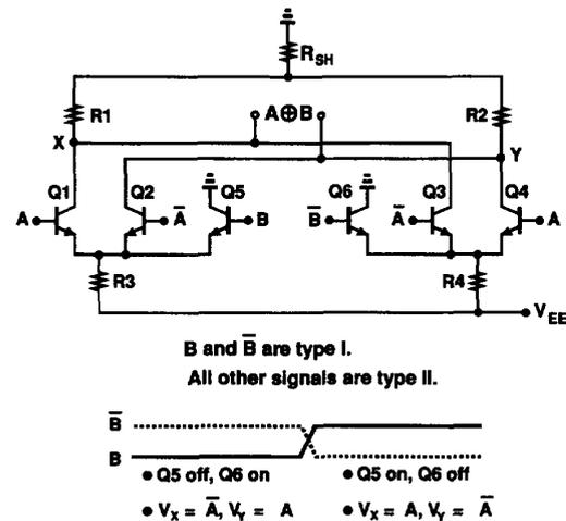
Fig. 5. Exclusive-OR gate derived from MUX of Fig. 3.
