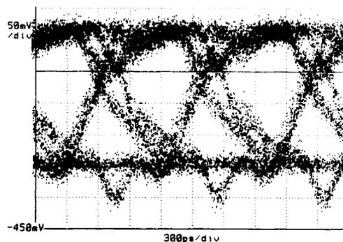
Fig. 16. Measured MUX output at 1 Gb/s.
