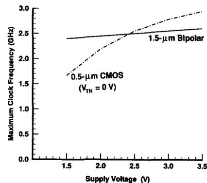
Fig. 12. Maximum clock frequency of bipolar and CMOS dividers versus supply voltage.
