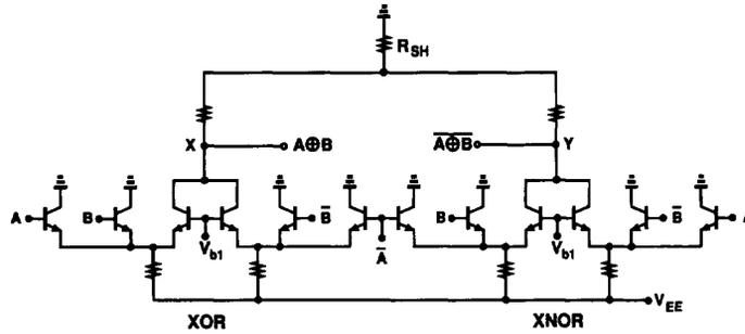
Fig. 7. Symmetric XOR gate with differential output.
