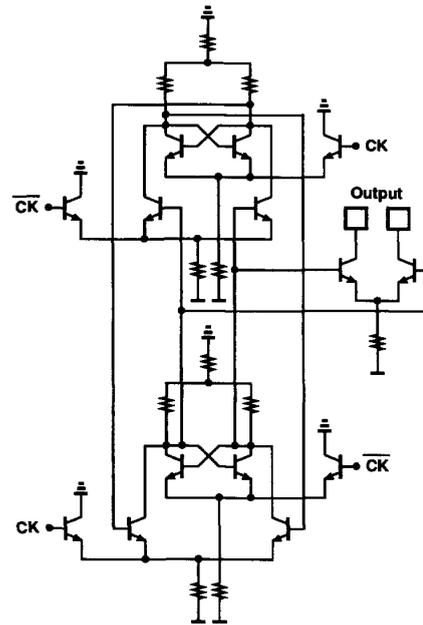
Fig. 10. Bipolar frequency divider.
