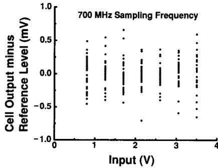
Fig. 9. Pedestals of all 32 cells in one channel as a function of input voltage after subtraction of the response to a reference input level. The nominal input value has been subtracted from the data. (Several data points are superimposed.)
