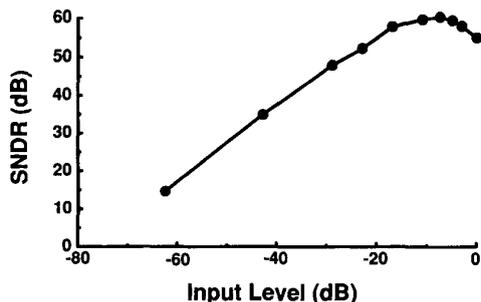
Fig. 12. Signal-to-(noise+distortion) ratio as a function of amplitude for a 21.4-MHz sine wave sampled at 700 MHz.
