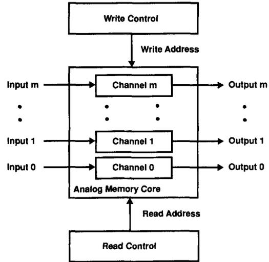
Fig. 1. Block diagram of an analog waveform recorder with  $m$  memory channels.
