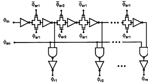
Fig. 5. Read control circuitry.
