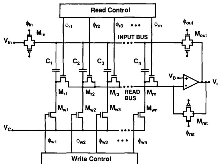
Fig. 2. Simplified schematic of the analog memory circuit.
