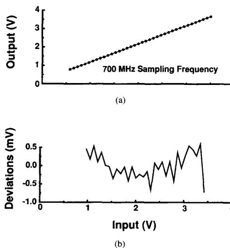
Fig. 8. (a) Output plotted as a function of input voltage for a 3-V input range. (b) Deviations from a linear fit for a 2.5 V input voltage range.
