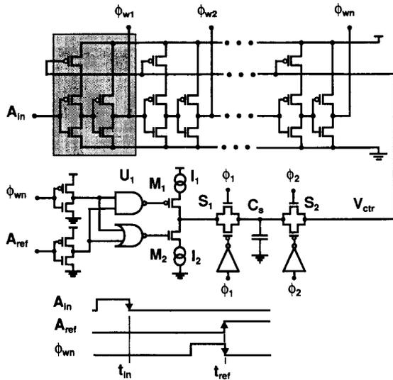
Fig. 4. Write control circuit with starved inverter delay elements and feedback compensation circuit.
