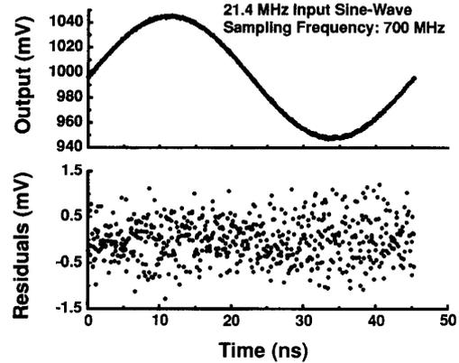
Fig. 11. Upper: Results of 20 measurement sets fitted to a 21.4-MHz sine wave and plotted on a time scale modulo the period of the sine wave. Lower: Residuals from the fit.
