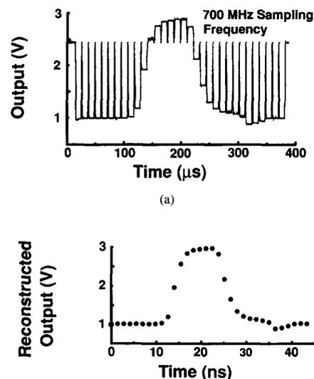
Fig. 7. Response of one channel to a 2-V input voltage step with a 3-ns rise-time sampled at 700 MHz. Pulse is plotted on (a) read and (b) write time scales.
