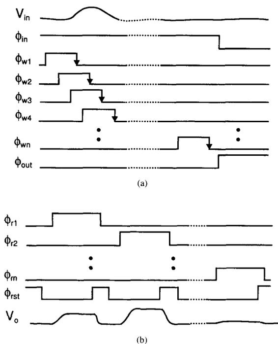
Fig. 3. Timing diagram for the (a) write and (b) read phases.
