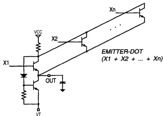
Fig. 5. Emitter-dotting of FPD-EF requires collectors of the emitter-follower transistors to be connected with an additional wire.
