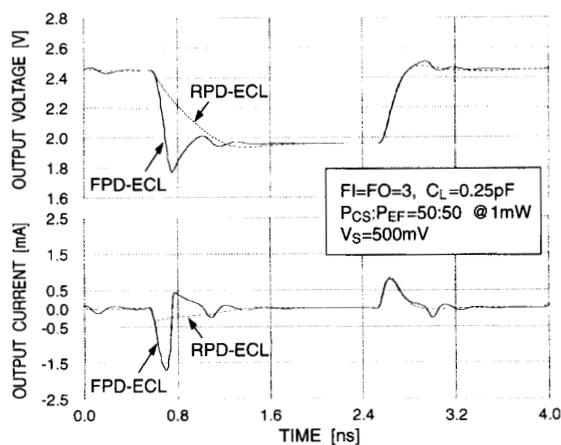
Fig. 8. Output waveforms and currents for loaded RPD and FPD ECL gates.
