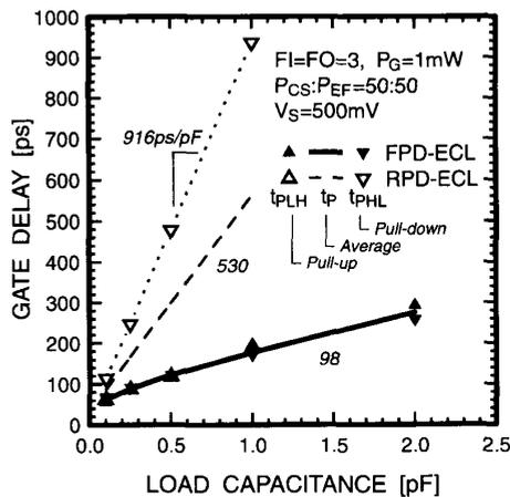
Fig. 10. Loaded gate delay versus load capacitance comparison between RPD and FPD ECL.
