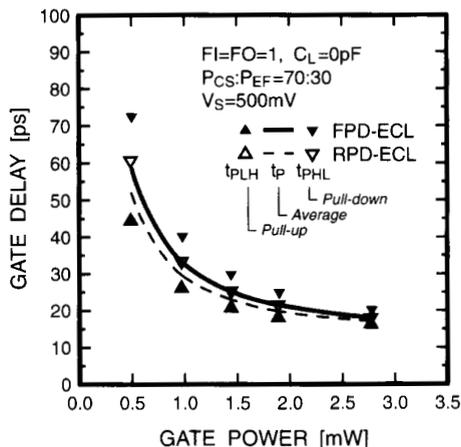
Fig. 6. Unloaded basic ECL ( $F_I = F_O = 1$ ,  $C_L = 0$ ) gate delay versus power consumption per gate comparison between RPD and FPD.
