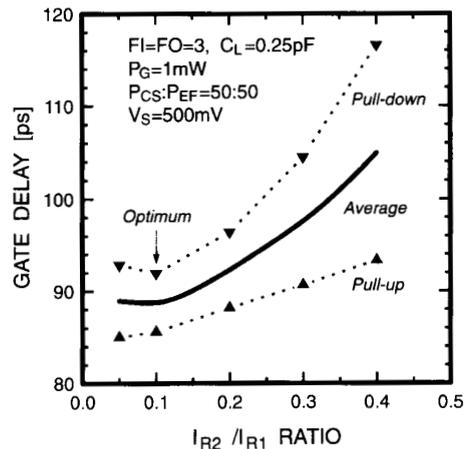
Fig. 7. Loaded FPD-ECL delay versus  $I_{R2}/I_{R1}$  current ratio.
