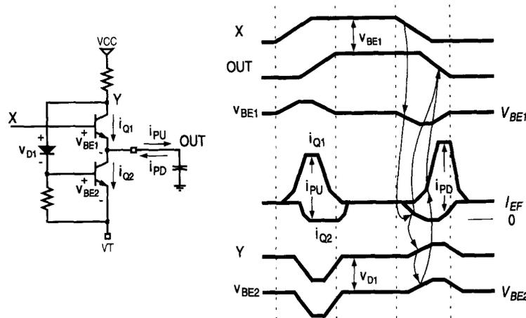
Fig. 4. Feedback-controlled push-pull operation of FPD-EF.
