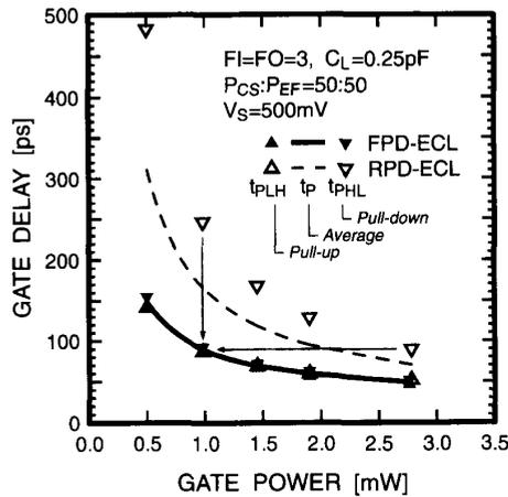
Fig. 9. Loaded ECL ( $FI = FO = 3, C_L = 0.25 \text{ pF}$ ) gate delay versus power consumption comparison between RPD and FPD.
