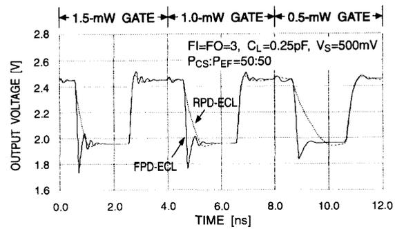
Fig. 11. Output ringing of loaded FPD-ECL gate ( $FI = FO = 3, C_L = 0.25 \text{ pF}$ ) for gate-power levels of 1.5, 1.0, and 0.5 mW compared with RPD-ECL.
