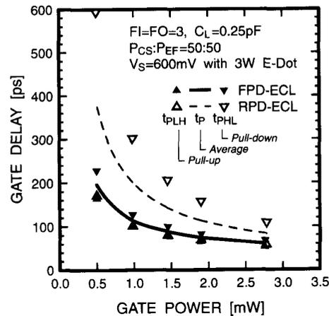
Fig. 12. Delay versus power consumption of 3-way emitter-dot gate with load compared between RPD and FPD ECL.
