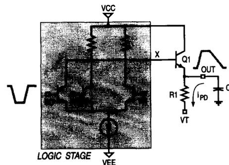
Fig. 1. Conventional resistor-pull-down (RPD) emitter follower (EF) for ECL/NTL.
