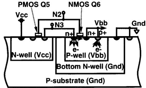
Fig. 8. Cross-sectional view of HPC with parasitic bipolar transistor.
