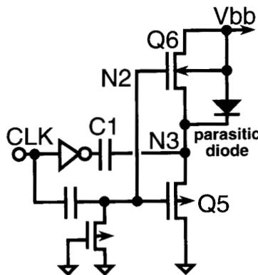
Fig. 5. Hybrid pumping circuit (HPC).
