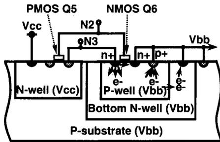
Fig. 7. Cross-sectional view of HPC.
