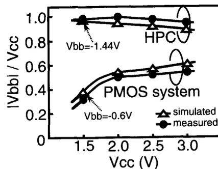
Fig. 11.  $V_{bb}$  level without load current.
