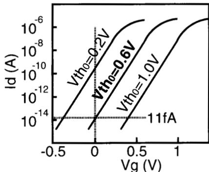
Fig. 3. Subthreshold characteristics of access transistor.
