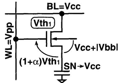
Fig. 1. Restoring operation.
