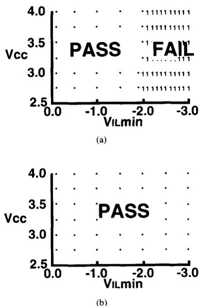
Fig. 10.  $V_{cc} - V_{IL\min}$  shmoo plot of test device. (a) Without triple-well. (b) With triple-well.
