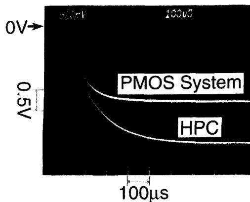
Fig. 13. Transient  $V_{bb}$  waveforms after power-on.
