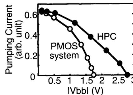
Fig. 12. Measured pumping current at  $V_{cc} = 3.0$  V.
