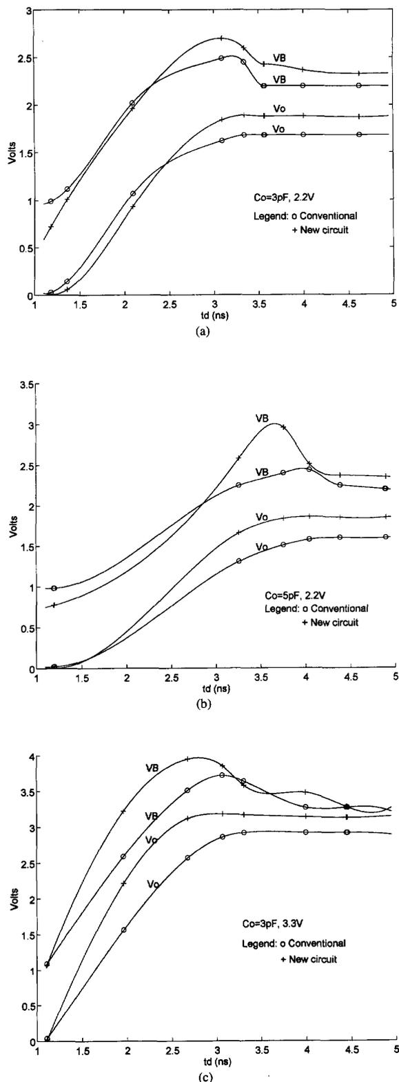
Fig. 3. Base voltage of  $Q_1$  and output rise response for conventional and new circuit. (a)  $C_0 = 3$  pF,  $V_{DD} = 2.2$  V, (b)  $C_0 = 5$  pF,  $V_{DD} = 2.2$  V, (c)  $C_0 = 3$  pF,  $V_{DD} = 3.3$  V  $\beta_{pnp} = 15$ .
