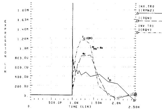
Fig. 7. The base current components of  $Q_2$ . ( $I_C$  of  $Q_n$  is shown for two values of  $W_{TN}$ ).  $\beta(Q_n) = 25$ .
