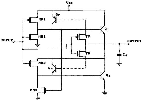
Fig. 1(c). BiCMOS buffer.
