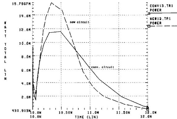
Fig. 11. Power dissipation in the new and conventional circuits (pull up), for  $C_0 = 3$  pF,  $V_{DD} = 3.3$  V, and  $f = 100$  MHz.
