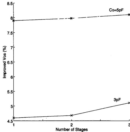
Fig. 10. Improved output voltage swing (in comparison with the conventional circuit) versus the number of stages for  $V_{DD} = 3.3$  V.
