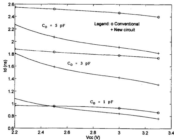
Fig. 6. The delay time of the new circuit of Fig. 1(b), compared to its conventional version for  $C_o = 5$  pF, 3 pF, and 1 pF.  $\beta_{pnp} = 15$ .
