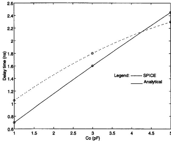
Fig. 9. Comparison between the rise time (analytical) and the delay time (SPICE) of the new circuit for  $V_{DD} = 2.2$  V,  $\beta(Q_p) = 15$ ,  $\beta(Q_n) = 25$ .
