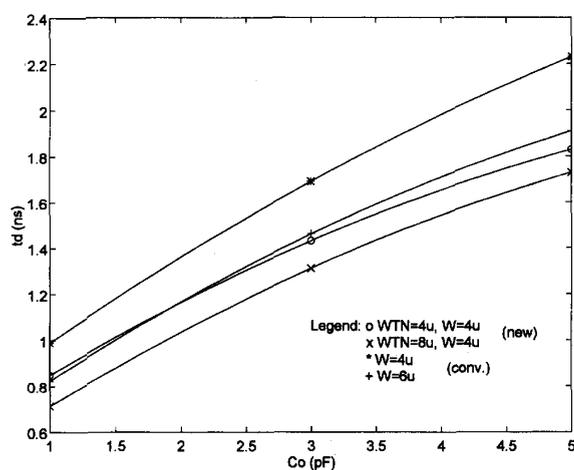
Fig. 8. The delay time of the pull down section of Fig. 1(c) for the new and conventional version.  $\beta(Q_n) = 25$ .
