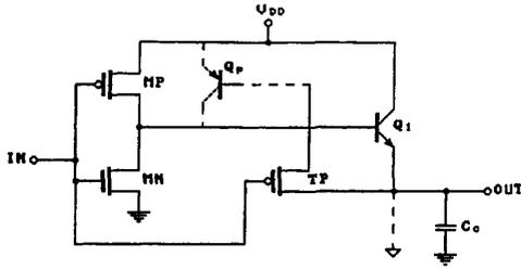
Fig. 1(a). BiCMOS pull up section.
