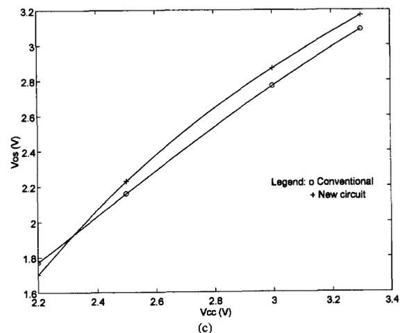
Fig. 5. Comparison of the output swing against the supply voltage between the new and conventional circuits. (a)  $C_0 = 5$  pF, (b)  $C_0 = 3$  pF, (c)  $C_0 = 1$  pF.  $\beta_{pnp} = 15$ .
