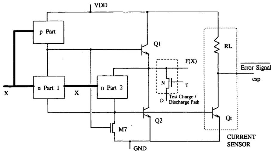
Fig. 3. Structure of a highly testable complex BiCMOS logic gate.
