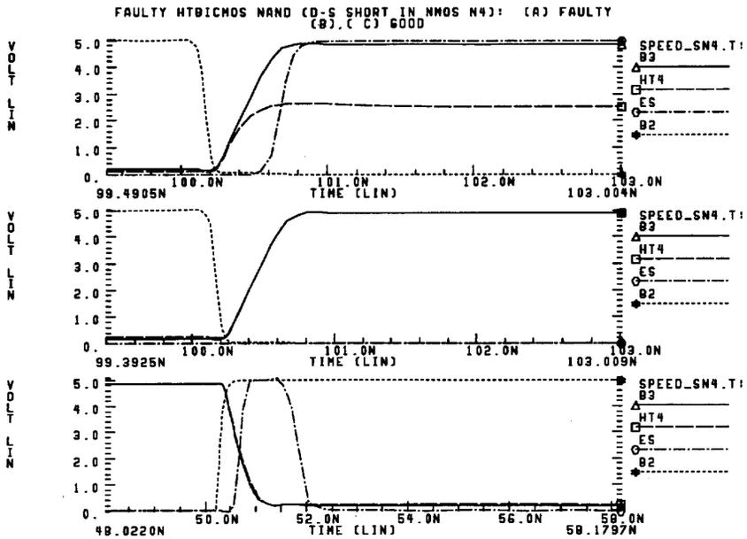
Fig. 9. Faulty *htnand* gate: shorted nMOS: (a) faulty gate, (b) good gate, (c) settling time for *es* (good gate).
