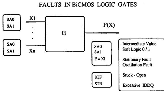
Fig. 2. Effects of shorts and opens on a BiCMOS logic Gate.
