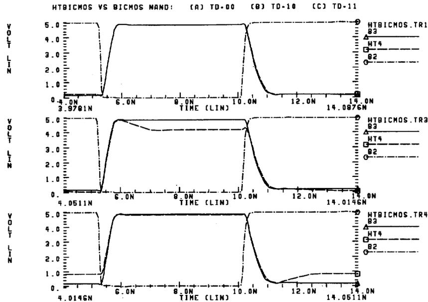
Fig. 7. Highly testable BiCMOS NAND (*htmand*) vs BiCMOS NAND Gate (*bnand*): (a)TD = 00, (b) TD = 01, (c) TD = 11.
