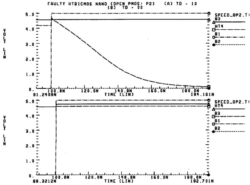
Fig. 8. Faulty *htnand* gate: open pMOS: (a) TD = 10, (b) TD = 00.
