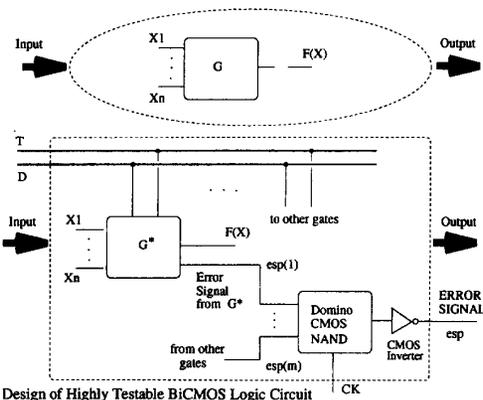
Fig. 5. Highly testable BiCMOS logic circuit design.
