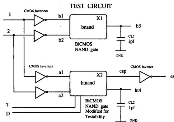
Fig. 6. Test circuit used to assess the performance and testability of the proposed design.
