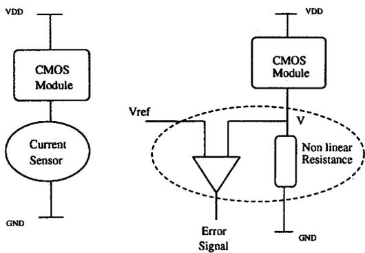
Fig. 4. CMOS built-in current sensing (BICS).
