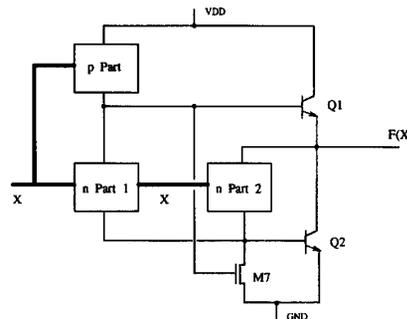
Fig. 1. General structure of a complex BiCMOS logic gate.
