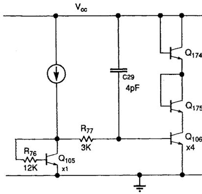
Fig. 7. Active supply bypass.
