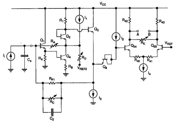
Fig. 3. Amplifier topology with variable-resistor MOSFET's included.
