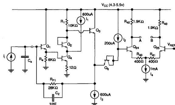
Fig. 1. Basic topology of the transimpedance amplifier in the high-gain condition.
