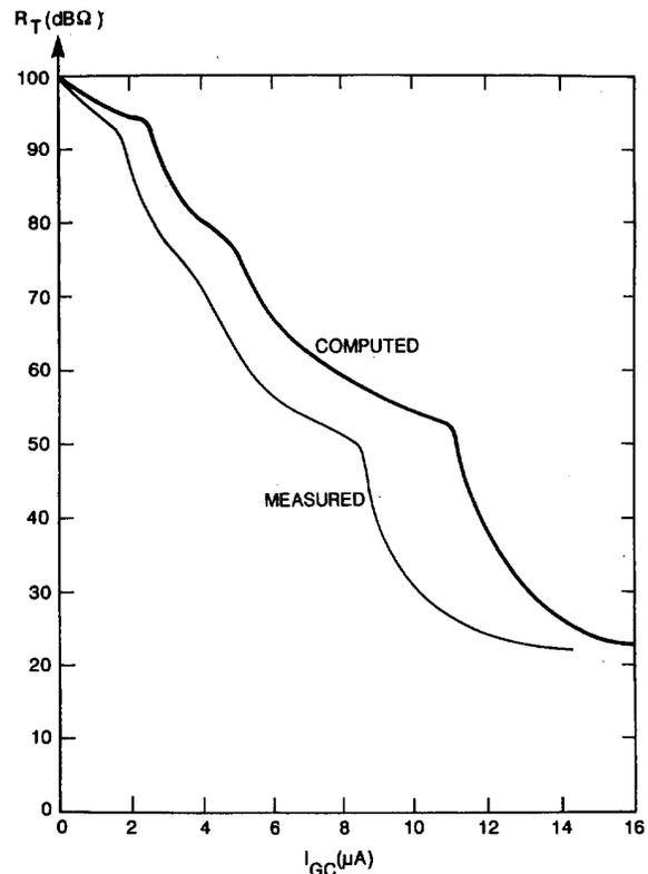
Fig. 9. Measured and computed transimpedance versus  $I_{GC}$ .
