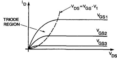
Fig. 4. MOSFET  $I_D - V_{DS}$  characteristics.
