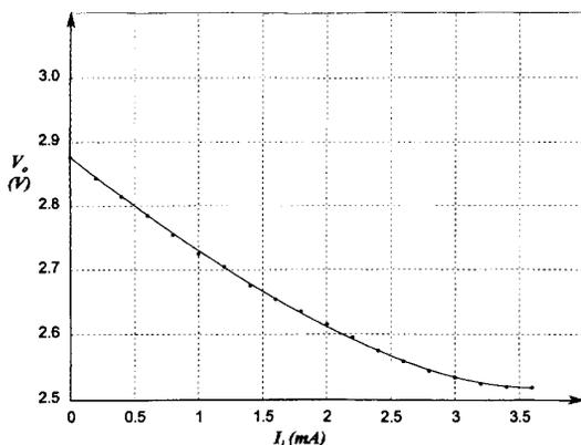
Fig. 11. Measured dc transfer 160 Ω characteristic at single-ended transimpedance.
