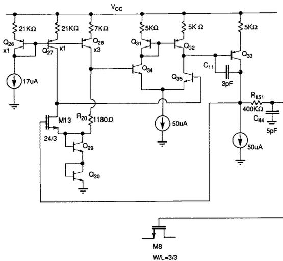
Fig. 5. Feedback amplifier setting the on-resistance of  $M_8$  as a multiple of precision resistor  $R_{20}$ .
