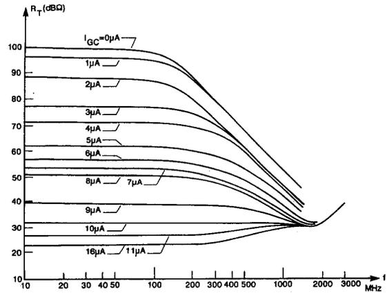
Fig. 8. Measured transimpedance versus frequency as a function of  $I_{GC}$ .
