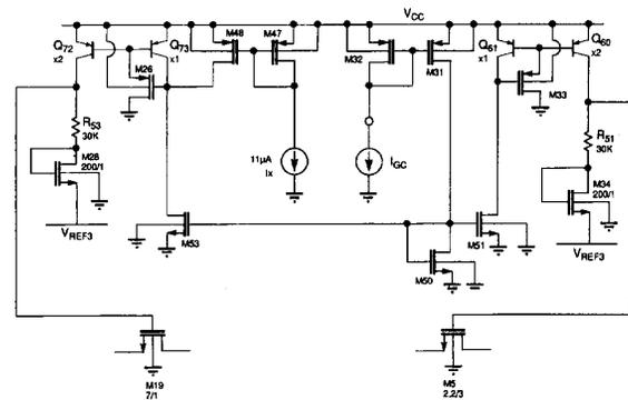
Fig. 6. Gain-control circuitry with precision gate-bias offsets for different variable-resistance MOSFET's.
