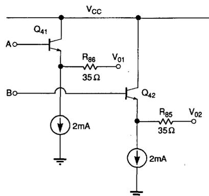
Fig. 2. Differential output stage.
