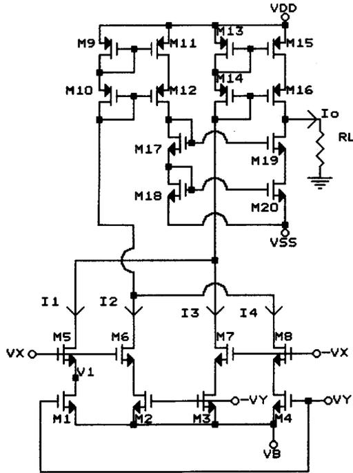
Fig. 1. The proposed four-quadrant multiplier circuit based on the bias feedback techniques.
