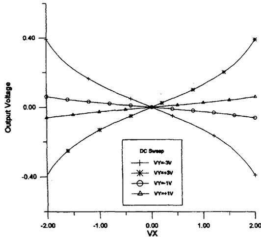
Fig. 3. The measured DC transfer functions of the proposed multiplier circuit with  $V_X$  changing from  $-3$  V to  $+3$  V and  $V_Y$  being equal to  $-3$  V,  $-1$  V,  $+3$  V, and  $+1$  V.
