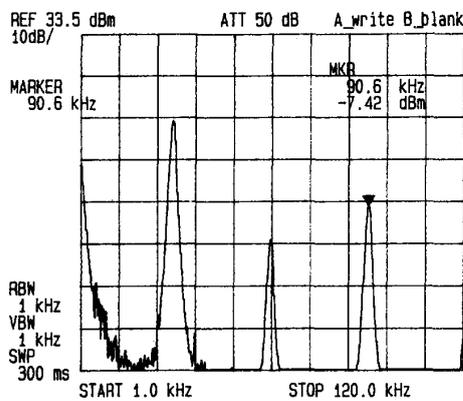
Fig. 4. A typical spectrum of the output voltage of the proposed multiplier. The vertical scale is 10 dBm/div.
