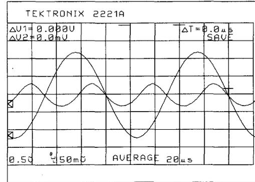
Fig. 5. The output waveform of the squaring circuit with a  $2.42$  V $_p$ - $_p$  sinusoidal input signal of  $10$  kHz. The horizontal scale is  $20$   $\mu$ s/div and the vertical scales are  $0.5$  V/div and  $50$  mV/div.
