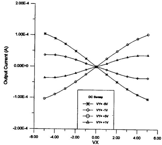
Fig. 2. The transfer characteristic curves of the proposed multiplier with  $V_Y = \pm 5 \text{ V}, \pm 1 \text{ V}$  and  $RL = 10 \text{ k}\Omega$ .  $V_X$  changes from  $-5 \text{ V}$  to  $5 \text{ V}$ .
