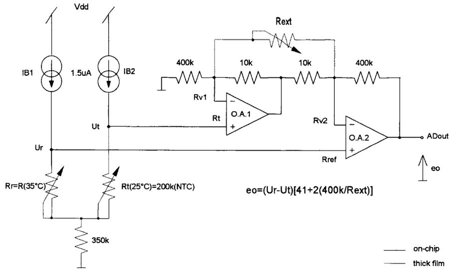
Fig. 2. The instrumentation amplifier for the temperature channels.
