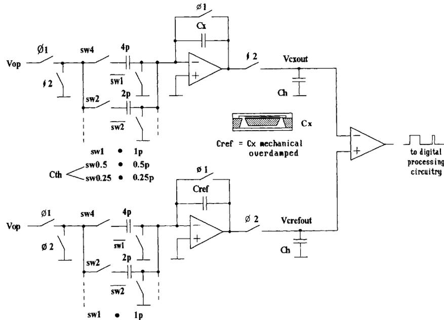
Fig. 3. The circuit diagram of the switched capacitor circuit.
