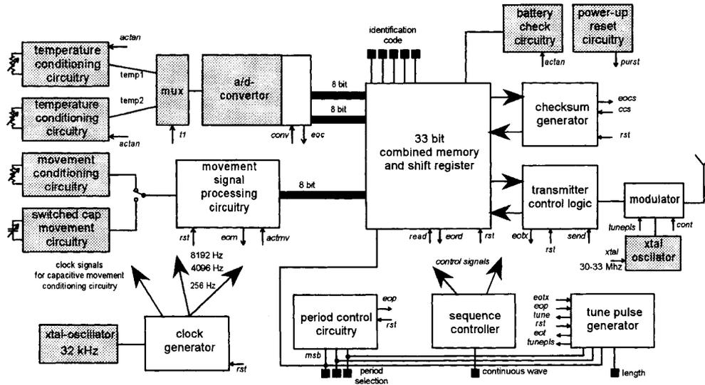
Fig. 1. The block diagram of the CMOS sensor interface chip.
