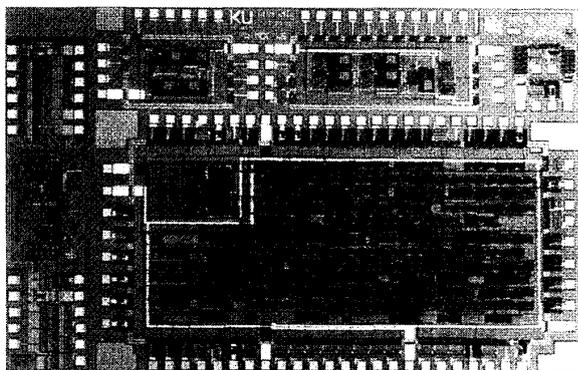
Fig. 5(a). Microphotograph of the CMOS sensor interface chip ( $4.7 \times 7.1 \text{ mm}^2$ ).
