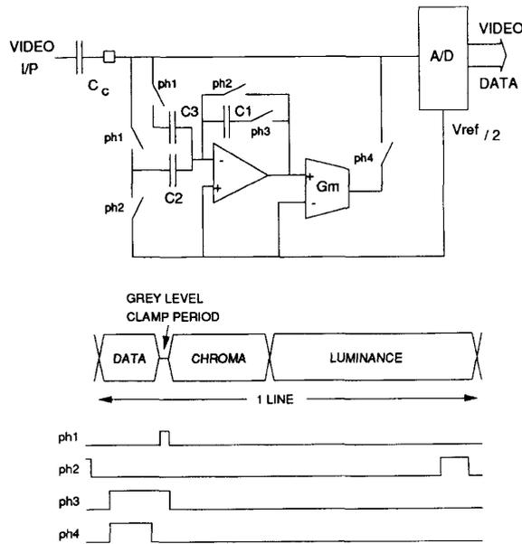
Fig. 5. Switched capacitor clamp circuit for satellite signals.
