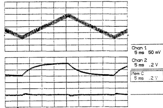
Fig. 6. Measured clamp circuit responses. Upper trace, free running triangle test signal applied via coupling capacitor, center trace, response at input pin of single pole clamp showing line-to-line offset, lower trace, response of two pole SC clamp circuit.
