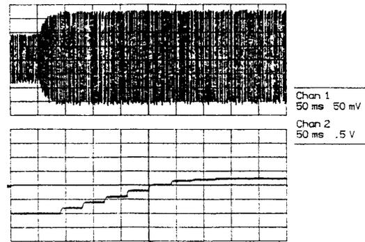
Fig. 4. Measured response of AGC to step in video envelope. Upper trace, video envelope, lower trace, voltage at top of A/D reference ladder.
