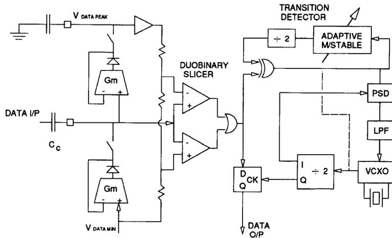
Fig. 7. Data signal path slicing and timing recovery structure.
