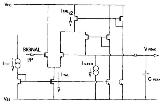
Fig. 8. Peak detector circuit.
