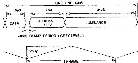
Fig. 1. D2-MAC signal structure, with dispersal signal.
