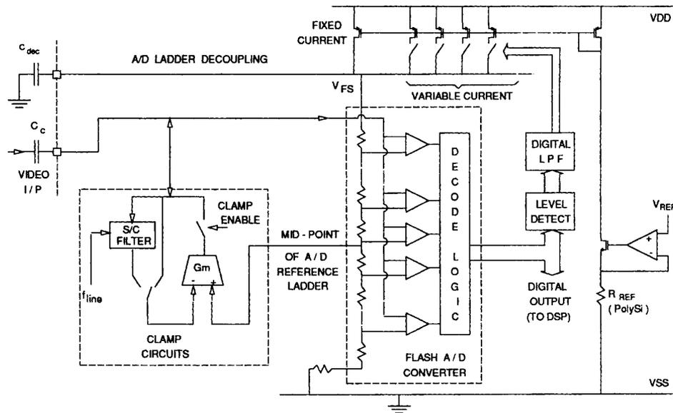
Fig. 2. Video signal path structure, showing AGC system. (Clamp circuits in terrestrial mode).
