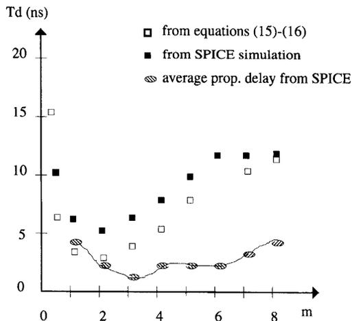
Fig. 4. Plot of  $T_d$  versus  $m$  from (15) and (16) and SPICE simulations. The average propagation delay,  $T_{pd}$ , obtained from SPICE simulations is also plotted.
