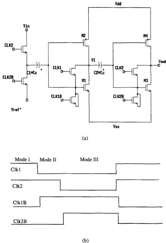
Fig. 2. a) Simplified schematic diagram of two-stage ac-coupled inverter chopper amplifier. b) Required timing diagram.
