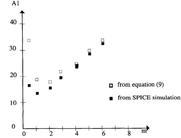
Fig. 3. Plot of  $A_1$  versus  $m$  from (9) and SPICE simulations.
