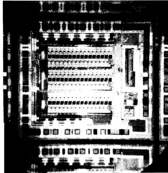
Fig. 6. The die photo of the 20 MHz triple 6-bit ADC chip.
