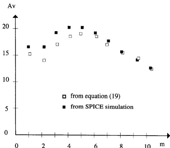
Fig. 5. Plot of  $A_v$  versus  $m$  from (19) and SPICE simulations.
