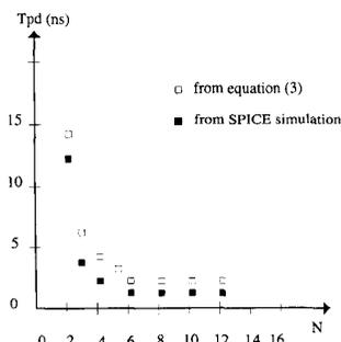
Fig. 1. Plot of  $T_{pd}$  versus  $N$  obtained from (3) and SPICE simulations with  $A_1 \gg 1$ .
