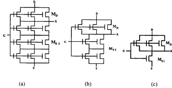
Fig. 2. Arrays of unit transistors with the same drain width ( $W_D = 3W_u$ ) and the same aspect ratio  $(W/L)_{eq} = 3/4$ . (a)  $(L/W)_{eq} = 3L_u/3W_u + L_u/3W_u$ , (b)  $(L/W)_{eq} = 2L_u/2W_u + L_u/3W_u$ . (c)  $(L/W)_{eq} = L_u/W_u + L_u/3W_u$ .
