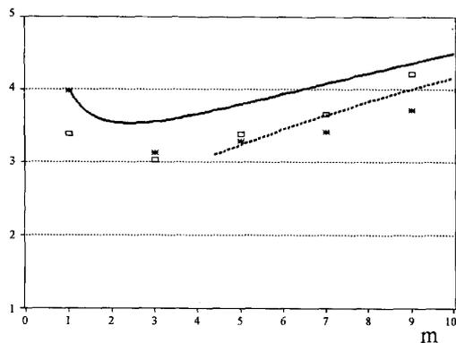
Fig. 11. Normalized transit time of the  $T_m$ -transistor ( $m$  is the number of parallel-connected transistors at the drain side): — theoretical; ---, asymptotic curve for high values of  $m$ ; □, experimentally determined at  $V_{GS} = -2$  V; \*, experimentally determined at  $V_{GS} = -3$  V.
