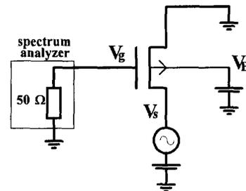
Fig. 9. Circuit to measure the gate-to-source capacitance.
