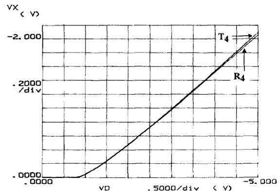
Fig. 6. Voltages at internal nodes  $X$  of the composite rectangular ( $R_4$ ) and trapezoidal ( $T_4$ ) transistors for  $V_D = V_G$ , with  $m$ , the number of parallel transistors at the drain side, equal to 4.
