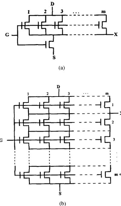
Fig. 4. Composite transistors: (a) Trapezoidal type composite transistor ( $T_m$ -transistor)  $(L/W)_{eq} = L_u/W_u + L_u/mW_u$ . (b) Rectangular type composite transistor ( $R_m$ -transistor)  $(L/W)_{eq} = mL_u/mW_u + L_u/mW_u$ .
