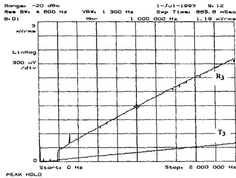
Fig. 10. Experimental results for the gate-to-source transadmittance in the rectangular ( $R_3$ ) and trapezoidal ( $T_3$ ) transistors  $V_{DB} = V_{GB} = -3$  V,  $V_{SB} = 0$  V.
