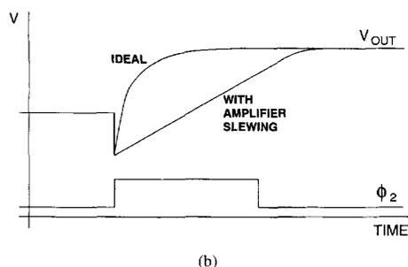
Fig. 1. (a) Switched-capacitor integrator and (b) the effect of slew rate on integrator transient response. If the slew rate is too low, the integrator will not settle before the end of the clock cycle.
