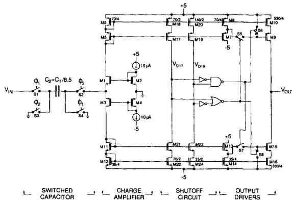
Fig. 3. Circuit diagram of booster circuit.
