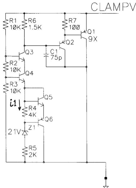
Fig. 3. Schematic diagram of 72-V high-current clamp circuit.
