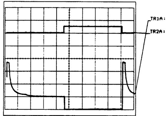
Fig. 4. Input/Output response of driver, with a 15- $\Omega$ , 18-mH load.  $TR2A = V_{input}$ , 10 V/div.  $TR1A = V_{out}$ , 20 V/div. Horizontal = 500  $\mu$ s/div.
