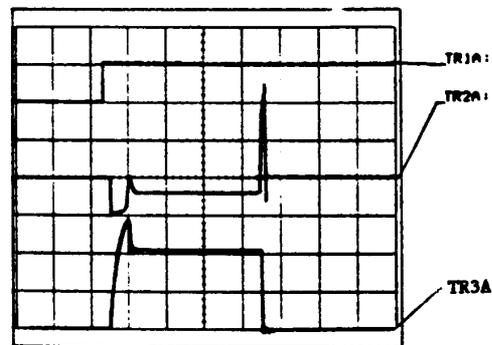
Fig. 6. Input/Output response of driver, with short inductive load, 4  $\Omega$  in series with 36  $\mu$ H.  $TR1A = V_{input}$ , 5 V/div.  $TR2A = V_{out}$ , 20 V/div.  $TR3A =$  output current, 1A/div. Horizontal = 50  $\mu$ s/div.
