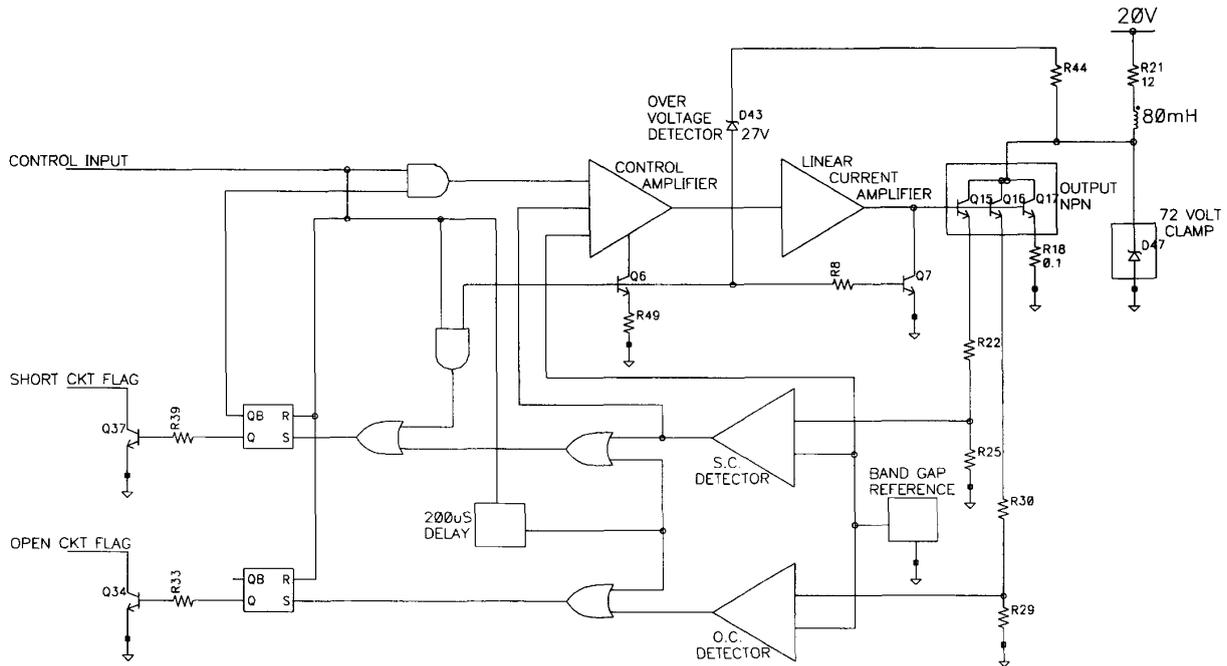
Fig. 1. Block diagram for high-voltage, high-current driver.
