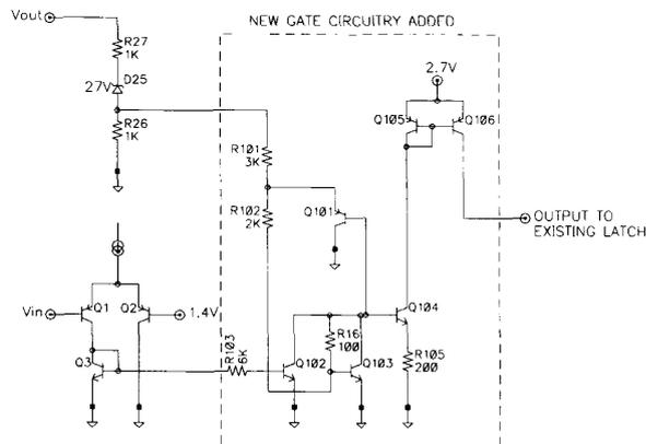
Fig. 2. Schematic diagram of gate circuit for over-voltage/over-current protection.
