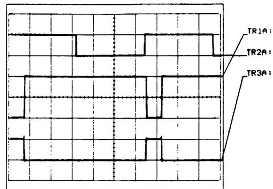
Fig. 5. Input/Output response of driver, with a 10- $\Omega$  load.  $TR2A = V_{input}$ , 5 V/div.  $TR1A = V_{out}$ , 10 V/div.  $TR3A =$  short-circuit flag, 5 V/div. Horizontal = 200  $\mu$ s/div.
