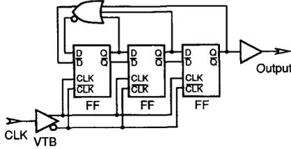
Fig. 9. 4-b counter block diagram.
