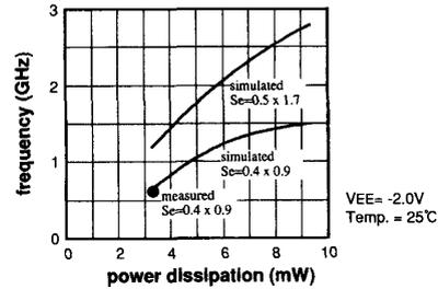
Fig. 11. Maximum operating frequency of 4-b counter.
