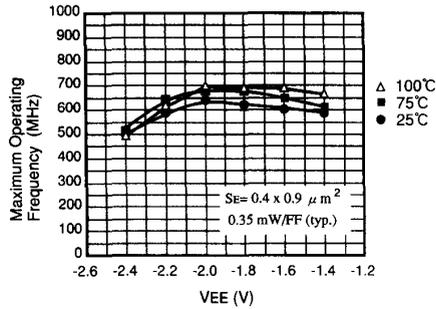
Fig. 10. Operating frequency variation of 4-b counter versus  $V_{EE}$ .
