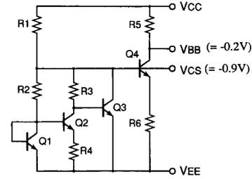
Fig. 4. Reference voltage generator.
