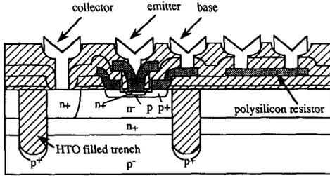
Fig. 6. Cross-sectional view of transistor.
