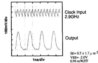
Fig. 12. Simulated wave form of 4-b counter.
