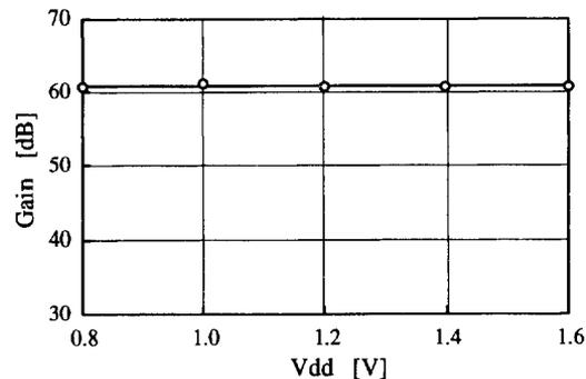
Fig. 14. Gain versus supply voltage.
