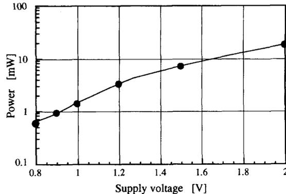
Fig. 20. Power consumption versus supply voltage.
