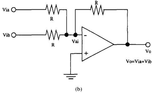
Fig. 11. Analog subtractor (a) and adder (b) circuits.
