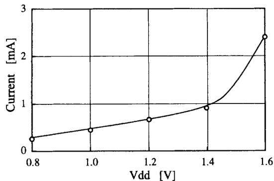
Fig. 16. Circuit current versus supply voltage.
