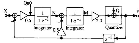
Fig. 6. Delta-sigma scheme in respect to the circuit noise.
