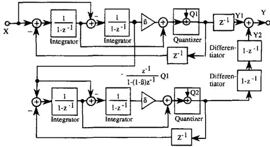
Fig. 9. Fourth-order cascade-connected swing-suppression scheme.
