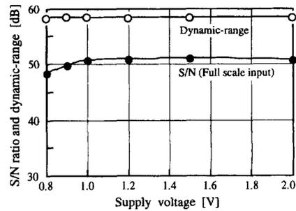
Fig. 19.  $S/N$  ratio and dynamic-range versus supply voltage.
