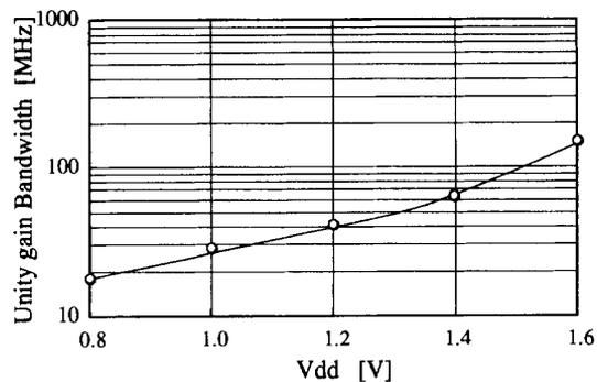
Fig. 15. Unity gain bandwidth versus supply voltage.
