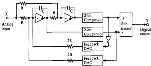
Fig. 10. Circuit blocks of the A/D converter.
