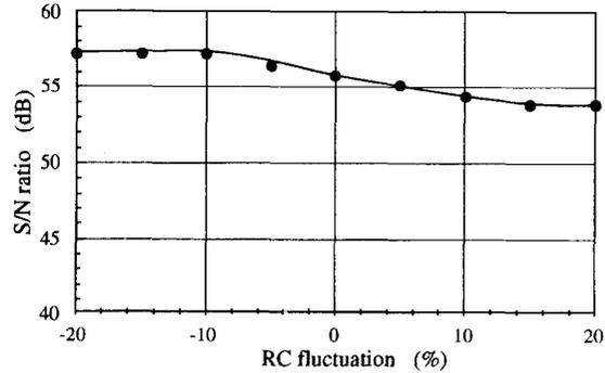
Fig. 7. Simulated  $S/N$  ratios versus  $RC$  fluctuation.
