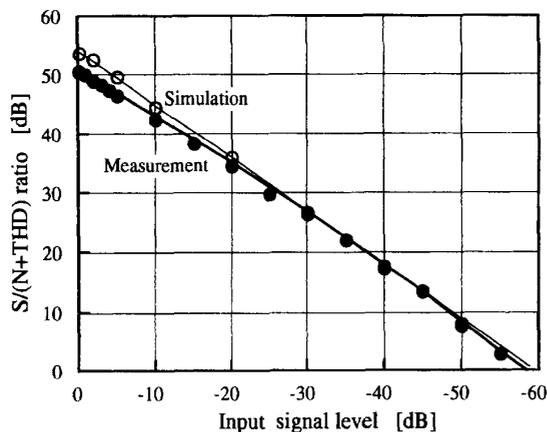
Fig. 18.  $S/N$  ratio versus input signal levels.
