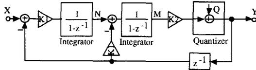
Fig. 4. Second-order delta-sigma scheme with scaling.
