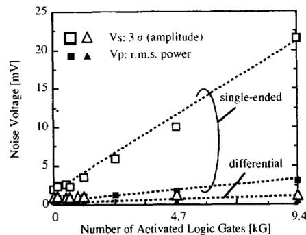
Fig. 9. Measured noise dependence on the number of activated logic gates.
