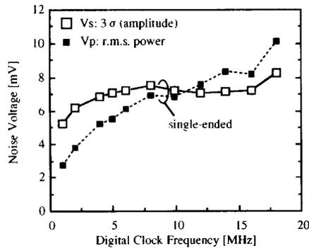
Fig. 10. Measured noise dependence on digital clock frequency.
