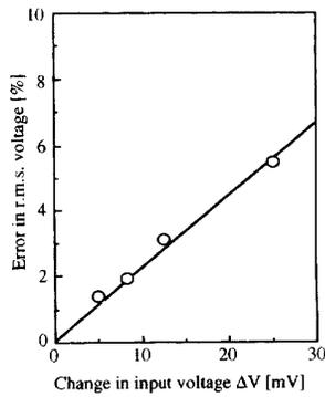
Fig. 3. Error in rms voltage dependence on  $\Delta V$ .
