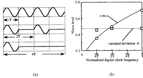
Fig. 5. Simulation results for standard deviation and rms voltage. (a) Simulated noise waveforms. (b) Simulated noise voltage.
