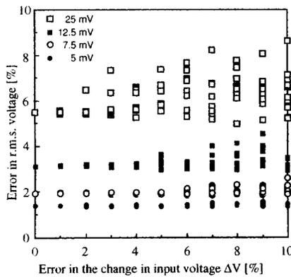
Fig. 4. Error in rms voltage dependence on error in  $\Delta V$ .
