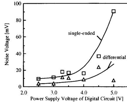
Fig. 11. Measured noise dependence on digital power supply voltage.
