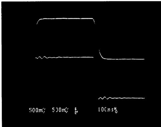
Fig. 4. 1 MHz 1.5  $V_{p-p}$  input signal. Top trace=output; bottom trace=input.
