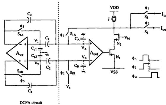
Fig. 1. Proposed CSH circuit with the differential clock feedthrough attenuation (DCFA) circuitry.
