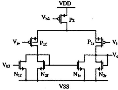
Fig. 2. The circuit diagram of the voltage buffer  $A_{buf}$  used in Fig. 1.
