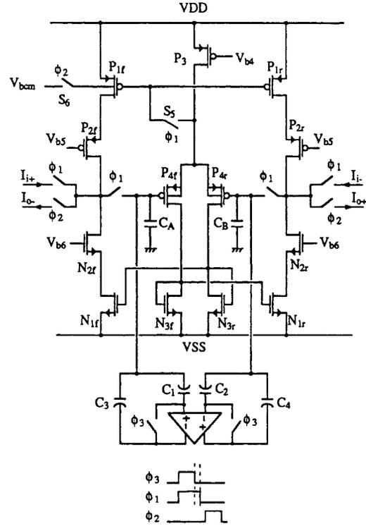
Fig. 3. The proposed fully differential dynamic-mirror CSH circuit.
