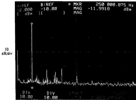
Fig. 8. Output spectrum of the CSH circuit for the 250 kHz, 410  $\mu\text{A}$   $p-p$  sinusoid input at 4 MHz clock rate.
