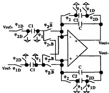
Fig. 14. Transmit SC filter 1 and 1 b DAC ( $B$  = modulator output bit).
