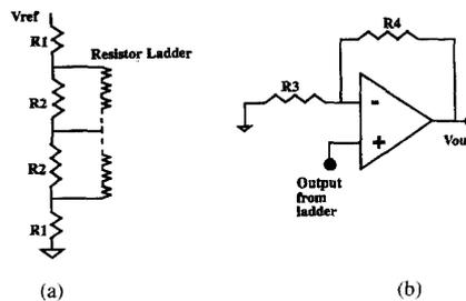
Fig. 17. Control DAC and output driver.
