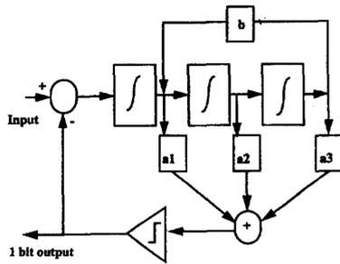
Fig. 4. Receive delta-sigma modulator.
