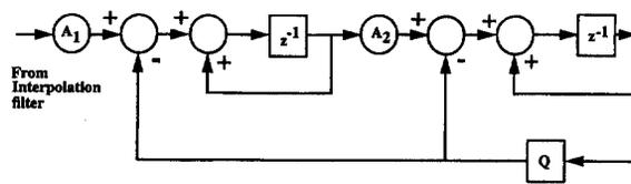
Fig. 13. Transmit digital delta-sigma modulator.
