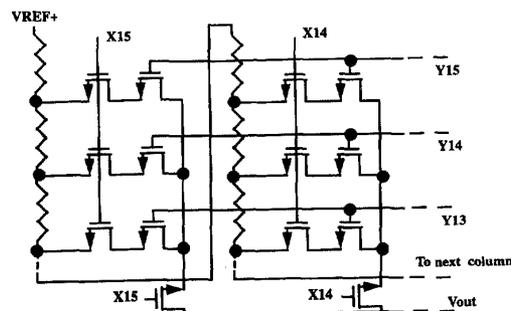
Fig. 18. Control DAC resistor ladder.
