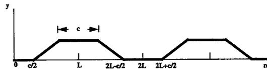
Fig. 20. Trapezoidal waveform.
