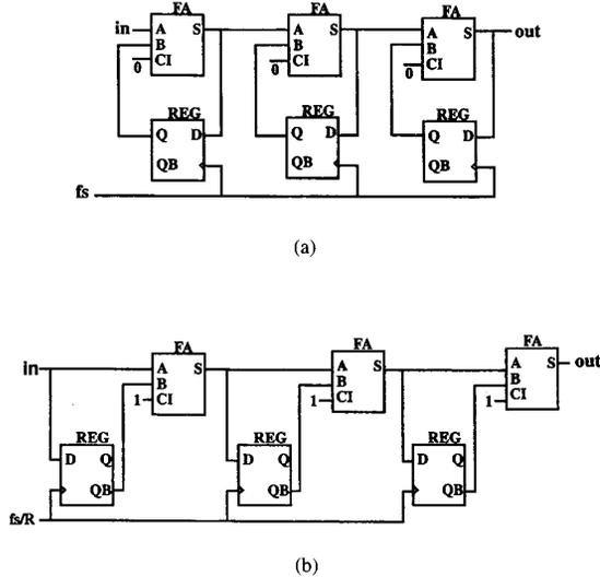
Fig. 8. Integrator and differentiator sections (FA = full adder, REG = register). (a) Integrator section. (b) Differentiator section.
