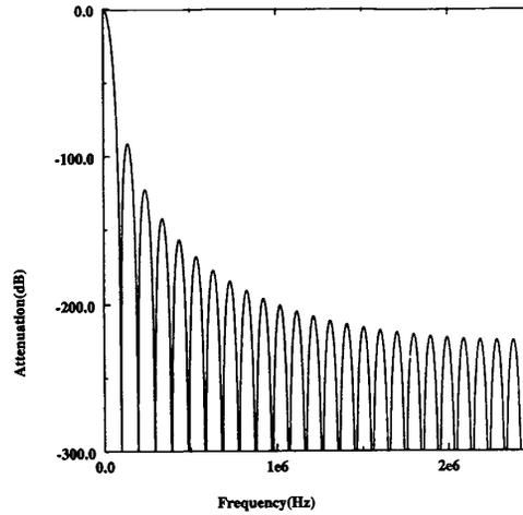
Fig. 10. Receive digital frequency response.
