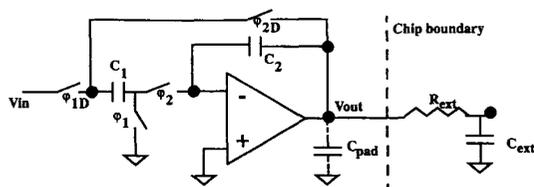
Fig. 15. Transmit SC filter 2 (single-ended version).
