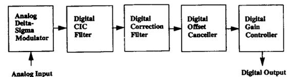
Fig. 3. Receive block diagram.
