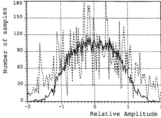
Fig. 2. Histogram of the integrator outputs. Dashed line—the first integrator output; Solid line—the second integrator output.
