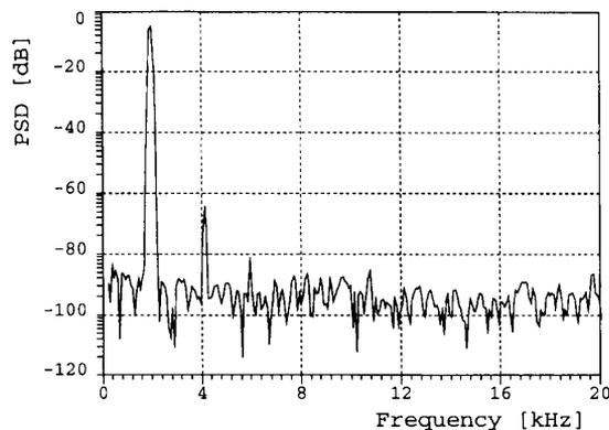
Fig. 7. Measured power spectrum. The clock frequency is 2.45 MHz and the input is a 2-kHz  $3.5\text{-}\mu\text{A}$  ( $-5.4\text{ dB}$ ) sinusoidal.
