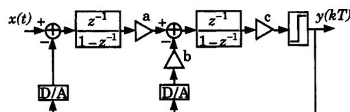
Fig. 1. Modulator structure.
