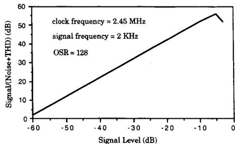
Fig. 8. Measured signal/(noise + THD) versus the input current. And the 0-dB signal level is  $6.5\text{ }\mu\text{A}$ .
