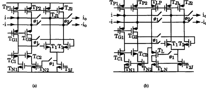
Fig. 3. (a) Conventional fully differential SI memory cell and, (b) low-voltage fully differential SI memory cell.
