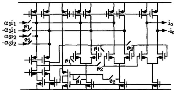
Fig. 4. Fully differential lossless integrator with CMFB.
