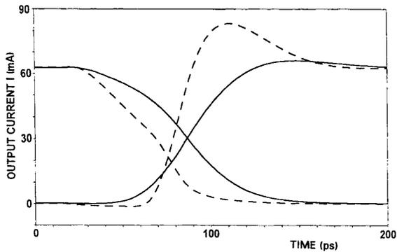
Fig. 8. Output current  $I$  for switching-on and switching-off using standard current source for  $v_{in} = 2 \times 170 \text{ mV}_{pp}$  (solid lines) and  $2 \times 500 \text{ mV}_{pp}$  (dashed lines).
