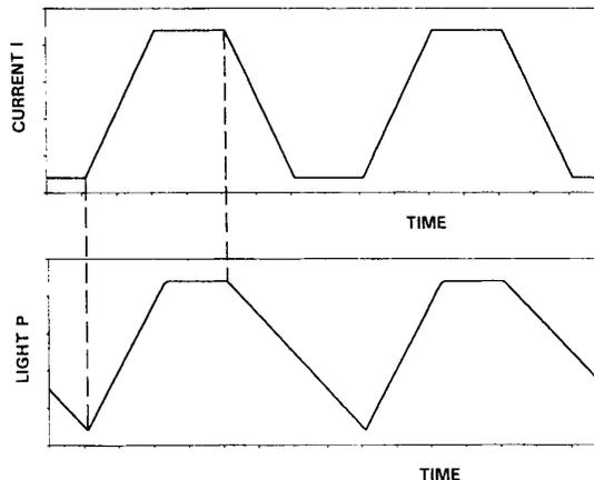
Fig. 1. Driving current and optical output power of a laser diode (schematically).
