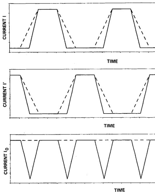
Fig. 6. Currents  $I$  and  $I'$  (see Fig. 3(a)) for constant (dashed lines) and switched (solid lines) current source (schematically).
