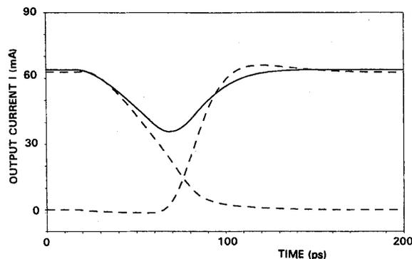
Fig. 11. Output current  $I$  for switching-on and switching-off using switched current source and  $v_{in} = 2 \times 500 \text{ mV}_{pp}$  (dashed lines). Solid line: current of the current source.
