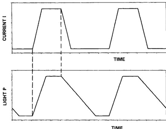
Fig. 4. Improved pulse shape of driving current and resulting optical output power of a laser diode (schematically).
