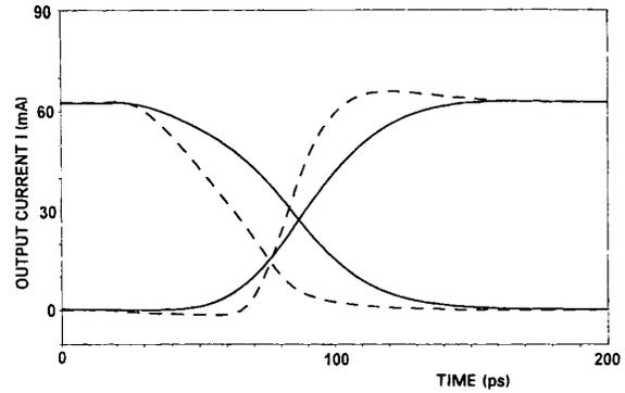
Fig. 9. Output current  $I$  for switching-on and switching-off using *switched* current source for  $v_{in} = 2 \times 170 \text{ mV}_{pp}$  (solid lines) and  $2 \times 500 \text{ mV}_{pp}$  (dashed lines).
