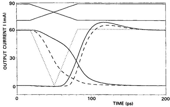
Fig. 7. Output current  $I$  for switching-on and switching-off for realistic current-switch transistors and *ideal* current sources: Constant current (solid lines) and switched current (dashed lines). Dotted line: Current of the switched current source. For reference, the corresponding input voltage  $v_{in}$  is sketched in the upper part.
