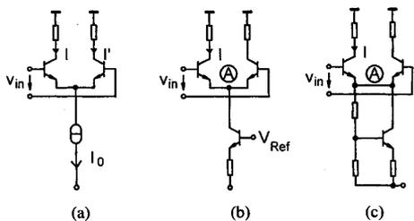
Fig. 3. Current switch with (a) ideal current source  $I_0$ , (b) standard transistor current source, (c) novel switched transistor current source.
