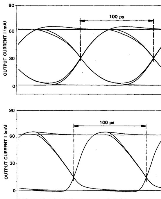
Fig. 12. Comparison of eye patterns of output current  $I$  for 10 Gb/s using standard (upper part;  $v_{in} = 2 \times 170 \text{ mV}_{pp}$ ) and switched (lower part;  $v_{in} = 2 \times 500 \text{ mV}_{pp}$ ) current source, respectively.
