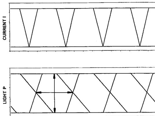
Fig. 5. Eye patterns for driving current and optical output power of a laser diode in the case of the improved shape of the driving current (schematically).
