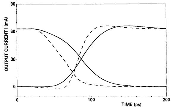
Fig. 10. Comparison of output current  $I$  for switching-on and switching-off for same overshoot using standard (solid lines;  $v_{in} = 2 \times 170 \text{ mV}_{pp}$ ) and switched current source (dashed lines;  $2 \times 500 \text{ mV}_{pp}$ ), respectively.
