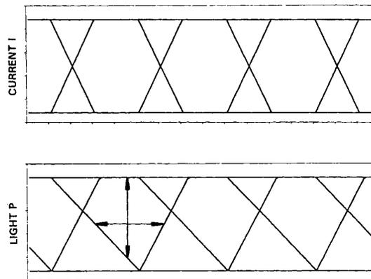
Fig. 2. Eye patterns for driving current and optical output power of a laser diode (schematically).
