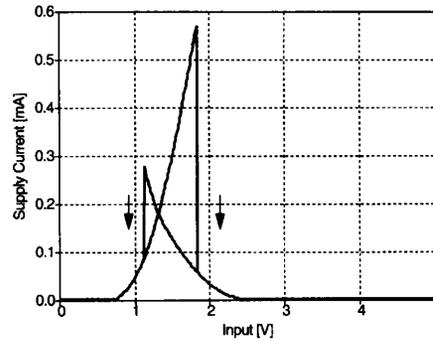
Fig. 7. Measured through-current as a function of the input voltage of the proposed input buffer. When the input voltage is larger than 2.4 V or smaller than 0.75 V, there is no through-current, and thus no static power consumption.
