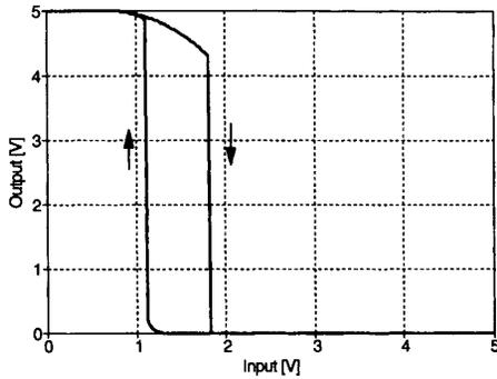
Fig. 6. The measured voltage transfer characteristic of the proposed input buffer shown in Fig. 3. The high-to-low and low-to-high logic threshold voltages are 1.83 and 1.11 V, respectively.
