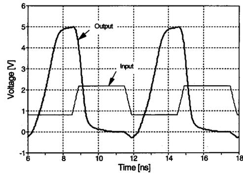
Fig. 10. Simulated transient response of the input buffer when driving a minimum sized inverter ( $W_N = 2 \mu\text{m}$ ,  $W_P = 6 \mu\text{m}$ ,  $L = 2 \mu\text{m}$ ) with the worst case TTL level; top trace—170 MHz input signal; bottom trace—output waveform.
