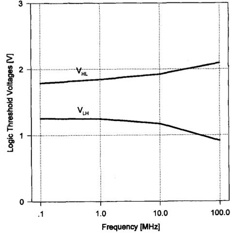
Fig. 4. The simulated dependency of the logic threshold voltages on the operating frequency.
