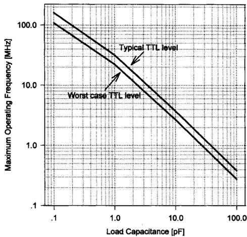
Fig. 9. Simulated dependency of the maximum operating frequency on the load capacitance.
