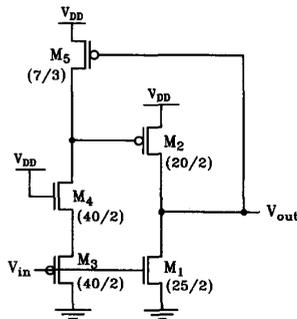
Fig. 3. The circuit diagram of the proposed TTL-to-CMOS input buffer. The (W/L) ratio of each transistor is shown in the parenthesis.
