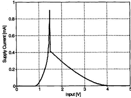
Fig. 2. Simulated through-current as a function of the input voltage of the conventional TTL-to-CMOS input buffer shown in Fig. 1. Through-current flows from  $V_{DD}$  to ground when the input lies between 0.8 V and 4 V, and thus there is large static power consumption.
