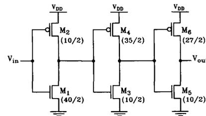
Fig. 1. Conventional TTL-to-CMOS input buffer. The (W/L) ratio of each transistor is shown in the parenthesis.
