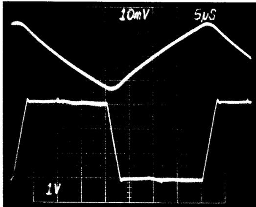
Fig. 8. High frequency square wave response with inductor.
