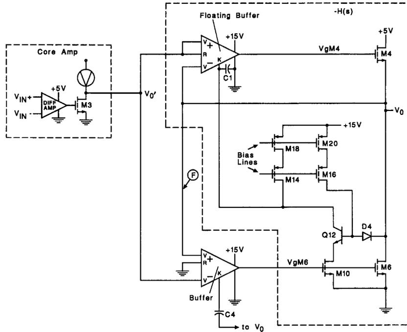
Fig. 3. Detailed amplifier system.
