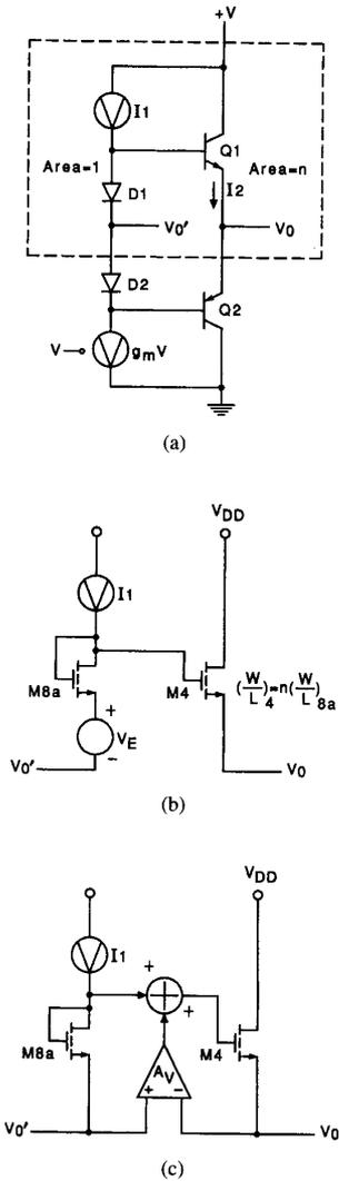
Fig. 1. Floating buffer derivation.
