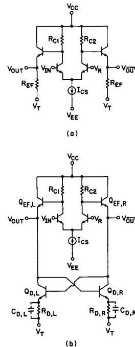
Fig. 1. Schematics of (a) conventional dual-phase ECL circuit, and (b) cross-coupled active-pull-down ECL (CC-APD-ECL) circuit.
