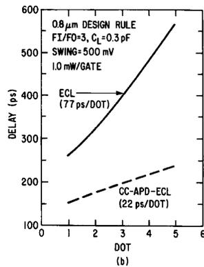
Fig. 7. (a) Schematics of 2-way output OR (emitter) dot using the CC-APD-ECL circuit, and (b) delay versus dot for the conventional ECL circuit and the CC-APD-ECL circuit. Notice that Dot = 1 equals no dotting. ( $0.8 \mu\text{m}$  design rule,  $FI/FO = 3$ ,  $1.0 \text{ mW/gate}$ ).
