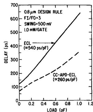
Fig. 6. Delay versus capacitive loading for the conventional ECL circuit and the CC-APD-ECL circuit. ( $0.8 \mu\text{m}$  design rule,  $FI/FO = 3$ , 1.0 mW/gate).
