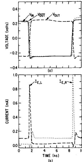
Fig. 3. Pertinent waveforms during the switching transient for the CC-APD-ECL circuit (refer to Fig. 1(b)): (a) voltage waveforms:  $V_{IN}$  is the input voltage,  $V_{OUT}$  and  $V_{OUT}$  are the out-of-phase and in-phase output voltage, respectively, and (b) current waveforms:  $I_{E,L}$  and  $I_{E,R}$  are the currents through the emitter-follower transistors  $Q_{EFL}$  and  $Q_{EFR}$ , respectively. (0.8  $\mu\text{m}$  design rule, FI/FO = 3,  $C_L = 0.3$  pF, 1.0 mW/gate).
