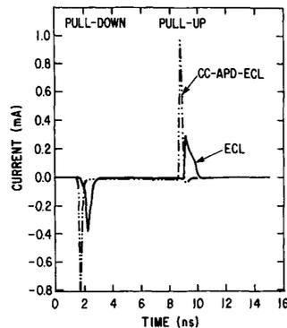
Fig. 2. Net pull-up and pull-down currents during the switching transient for the conventional ECL circuit and the CC-APD-ECL circuit. (0.8  $\mu\text{m}$  design rule, FI/FO = 3,  $C_L = 0.3$  pF, 1.0 mW/gate).
