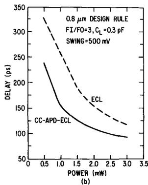
Fig. 4. (a) Unloaded ( $FI/FO = 1$ ) power-delay characteristics, and (b) loaded ( $FI/FO = 3$ ,  $C_L = 0.3$  pF) power-delay characteristics for the conventional ECL circuit and the CC-APD-ECL circuit at  $0.8 \mu\text{m}$  design rule.
