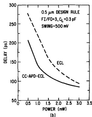
Fig. 5. (a) Unloaded ( $FI/FO = 1$ ) power-delay characteristics, and (b) loaded ( $FI/FO = 3$ ,  $C_L = 0.3$  pF) power-delay characteristics for the conventional ECL circuit and the CC-APD-ECL circuit at  $0.5 \mu\text{m}$  design rule.
