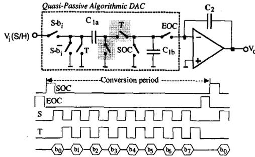
Fig. 1. (top) SC integrator employing a programmable positive SC branch with quasi-passive algorithmic DAC. (bottom) Switch timing.
