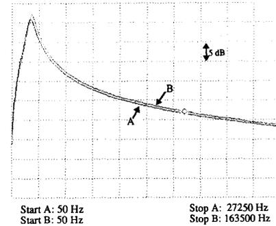
Fig. 9. Superimposed responses at  $F_s = 54.4$  kHz and  $F_s = 326$  kHz when the SC biquad is configured as a bandpass filter with 2 kHz pole frequency and  $Q = 5$ .
