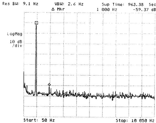
Fig. 10. Spectral contents of the output signal of the SC biquad, configured as a lowpass filter with 8 kHz pole frequency and  $Q = 1$ , when the test signal is a 1 kHz sinusoid with 2 V peak-to-peak.
