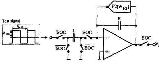
Fig. 6. SC biquad configured as a first-order lowpass filter for testing the linearity of the algorithmic DAC.
