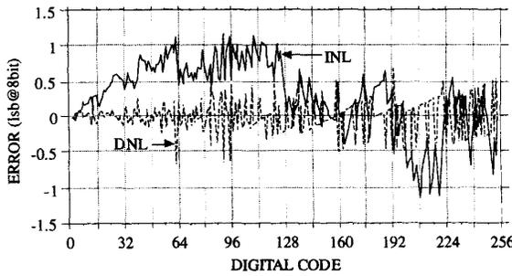
Fig. 7. INL and DNL characteristics of the programmable  $F_2$  SC branch.
