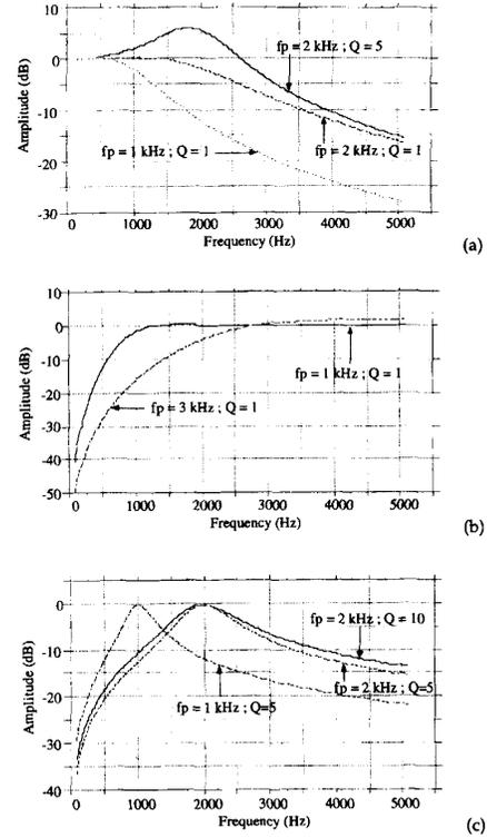
Fig. 8. Measured responses showing the programmability of the filtering shape, pole frequency and pole  $Q$ -factor. (a) Lowpass. (b) Highpass. (c) Bandpass.
