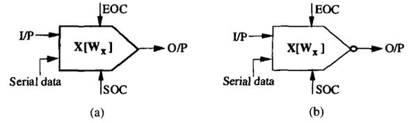
Fig. 2. Symbols representing the programmable (a) positive and (b) negative SC branches with quasi-passive algorithmic DAC's.
