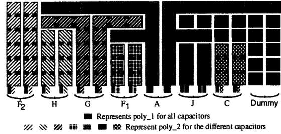
Fig. 4. Layout plan of the pairs of nominally equal capacitors in the programmable SC branches for matched grounded parasitic capacitances.
