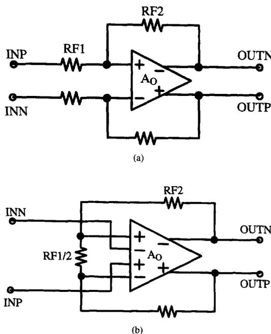
Fig. 1. Fully differential buffer amplifier topologies. (a) Inverting type. (b) Noninverting type.
