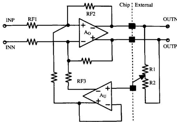
Fig. 2. Fully differential buffer with external gain control loop.
