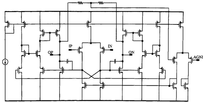
Fig. 9. Schematic of the core amplifier  $A_O$ .
