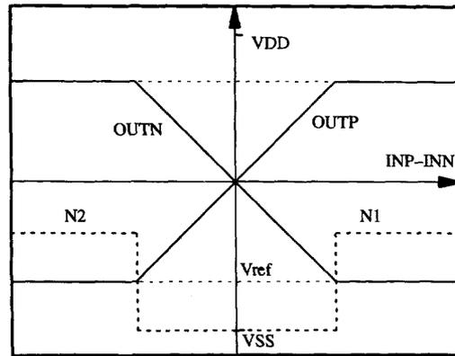
Fig. 8. DC transfer characteristic of the amplifier with clipping control.
