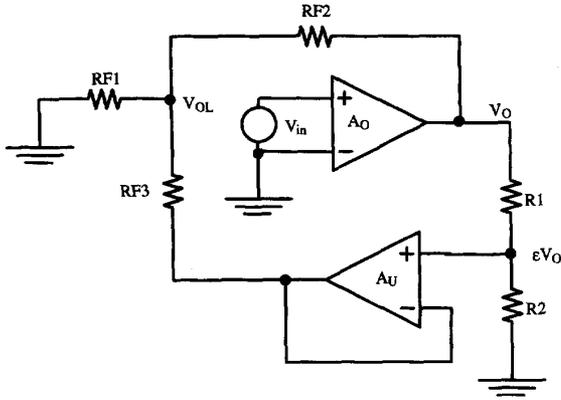
Fig. 5. Single-ended topology for stability analysis.
