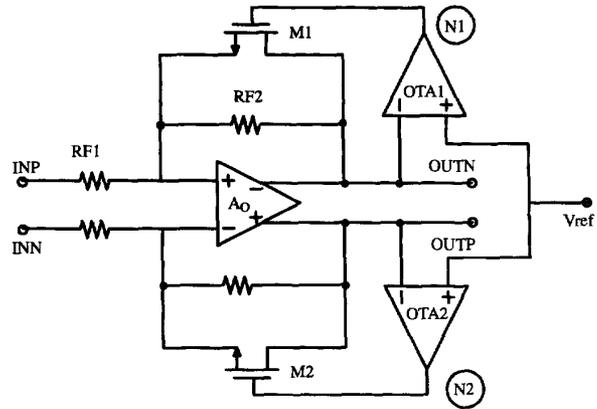
Fig. 7. Clipping control using a local feedback.
