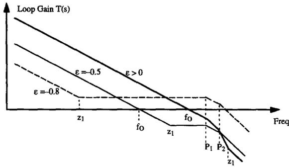
Fig. 6. Effect of the gain control loop on stability.
