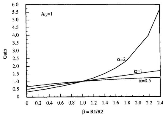
Fig. 3. Gain versus the external resistor ratio  $R_1/R_2$  for  $R_{F2}/R_{F1} = 1$ .
