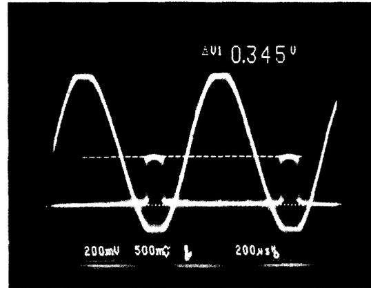
Fig. 11. Measured amplifier output signal with clipping control.
