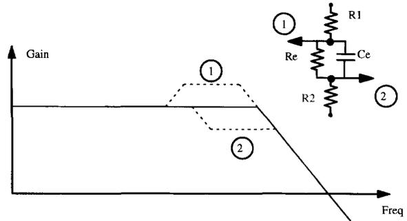
Fig. 4. Tunable transfer characteristic with external RC networks.
