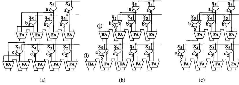
Fig. 2. Simplification of the carry ripple field multiplier.
