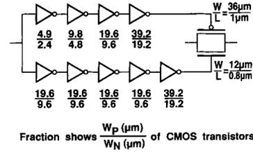
Fig. 9.  $\phi, \bar{\phi}$  signal generator for CMOS switch.
