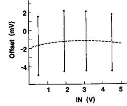
Fig. 13. Buffer amplifier offset standard deviation.
