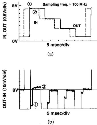
Fig. 14. ACC-SH dynamic waveforms. (a) ACC-SH input and output waveforms. (b) Difference between input and output waveforms.
