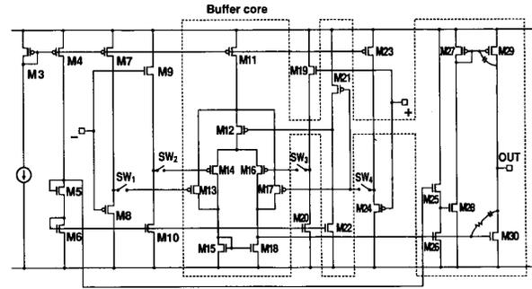
Fig. 10. Schematic diagram of the buffer amplifier.
