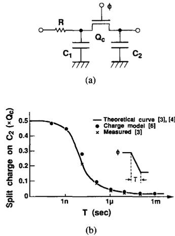
Fig. 5. Channel charge split phenomenon. (a) Test circuit. (b) Measured and simulated results.
