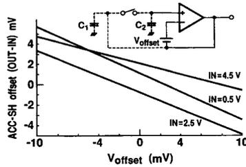
Fig. 12. Buffer  $V_{\text{offset}}$  effect simulation.
