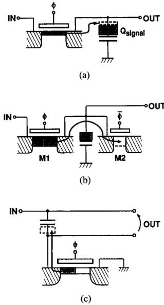
Fig. 2. Conventional S/H circuits. (a) Basic structure. (b) Use of compensation transistor. (c) Wooley's S/H circuit.
