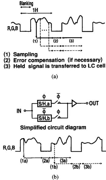
Fig. 3. The role of a S/H circuit for TFT-LCD. (a) Time schedule. (b) Actual time schedule.
