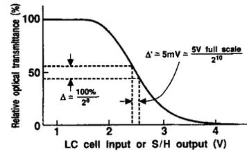
Fig. 4. Relative optical transmittance characteristics.
