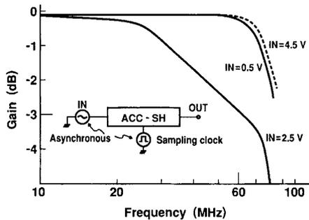
Fig. 15. ACC-SH offset frequency characteristics.
