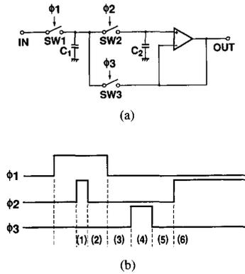
Fig. 6. ACC-SH. (a) Circuit diagram. (b) Switch control sequences, where 1) SW1 and SW2 are ON, both capacitors charge to IN, 2) SW2 turns OFF (SW1 is still ON),  $\frac{1}{2}$  SW2 charge is injected to  $C_2$ , 3) SW1 turns OFF,  $\frac{1}{2}$  SW1 charge is injected to  $C_1$ , 4) SW3 turns ON,  $V_{C_1}$  matches  $V_{C_2}$ , 5) SW3 turns OFF, leaving  $V_{C_1} \approx V_{C_2}$ , 6) SW2 turns ON,  $\frac{1}{2}$  SW1 charge on  $C_1$  returns to SW2.
