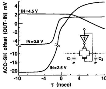
Fig. 8. Simulation of the effect of  $\tau$  on offset.
