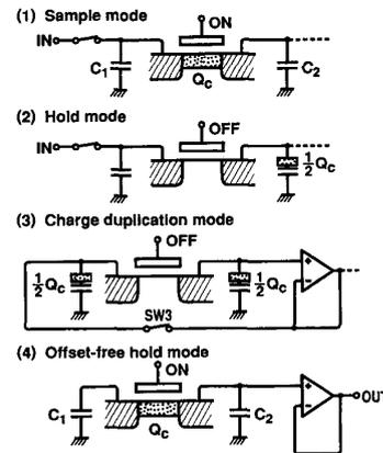
Fig. 7. ACC-SH operations to reduce the effect of channel charge.
