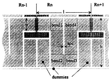
Fig. 2. Layout of basic resistor cell.
