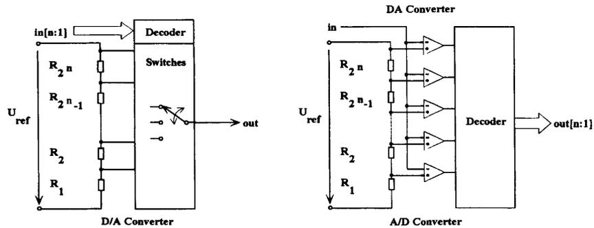
Fig. 1. Parallel resistor-string D/A and A/D converter.
