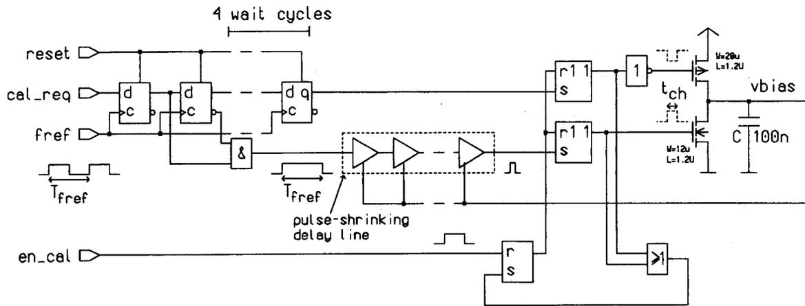
Fig. 7. Conceptual schematic of the delay-locked loop for delay stabilization.
