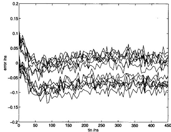
Fig. 12. Measured error due to temperature and supply changes. The error is the difference between the measured and the nominal value, which was measured with 5-V supply voltage at a temperature of  $+25^\circ\text{C}$ . The upper set of curves was measured with 4.5-V supply at temperatures of  $+60$ ,  $+40$ ,  $+10$ ,  $0$ ,  $-10$ ,  $-20$ , and  $-40^\circ\text{C}$ . The lower set of curves was measured with 5.5-V supply at the same temperatures.
