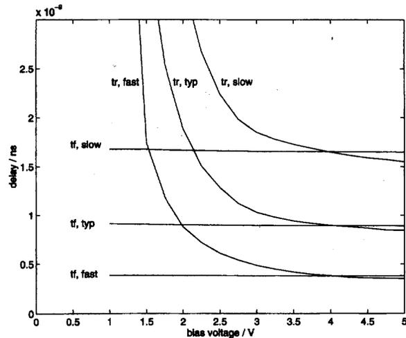
Fig. 6. Simulated propagation delays of the pulse-shrinking element for the rising ( $tr$ ) and falling ( $tf$ ) edge of the input pulse as a function of the bias voltage.
