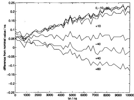
Fig. 13. Effect of temperature dependency of the oscillator on the measurement results at temperatures of  $+60$ ,  $+40$ ,  $+10$ ,  $0$ ,  $-10$ ,  $-20$ , and  $-40^\circ\text{C}$ . Nominal value was measured at the temperature of  $+25^\circ\text{C}$ .
