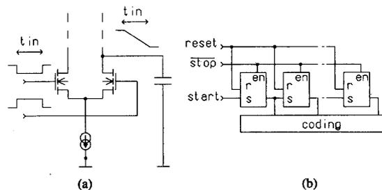
Fig. 3. Principle of (a) time-to-voltage conversion and (b) time interval measurement with a delay line.
