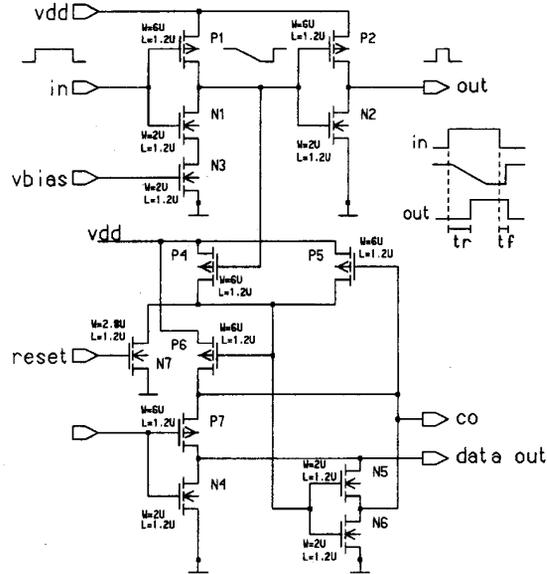
Fig. 5. Schematic diagram of the pulse-shrinking delay element.
