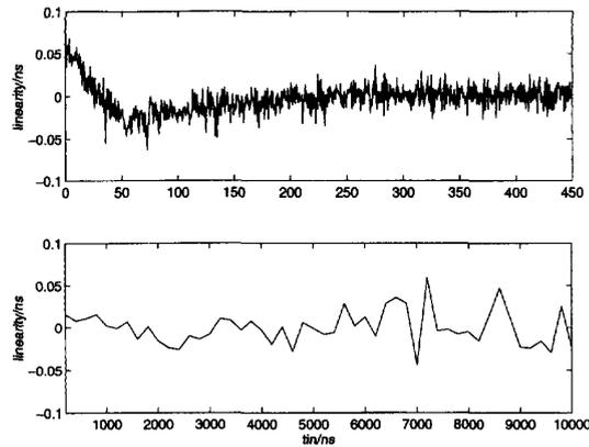
Fig. 11. Measured linearity of the TDC.
