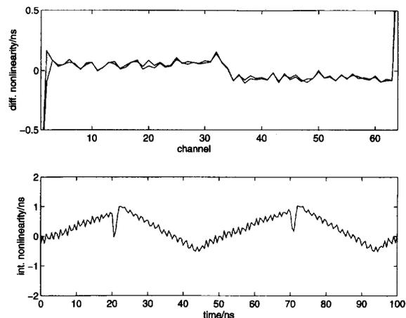
Fig. 10. Measured (top) differential nonlinearity of the two delay lines on one chip and (bottom) integral nonlinearity of one delay line.
