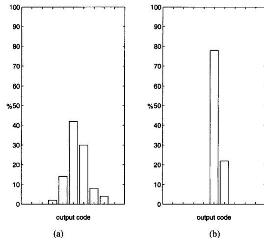
Fig. 9. Typical distribution of single-shot measurement results in 50 measurements. In (a), the input time interval is a multiple of half the clock period, and in (b), the input time interval is a multiple of the clock period.
