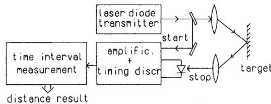
Fig. 1. Block diagram of the pulsed time-of-flight laser range-finder.
