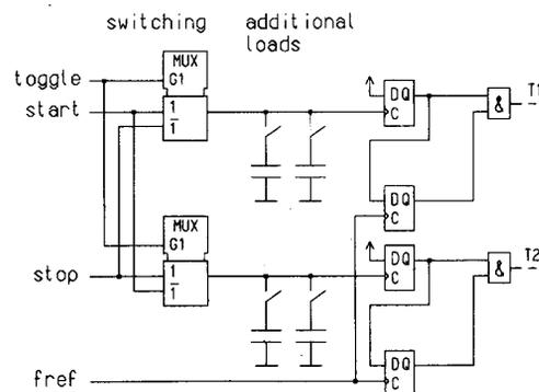
Fig. 8. Compensation of offset by adding extra load to start/stop channel or by switching start and stop channels.
