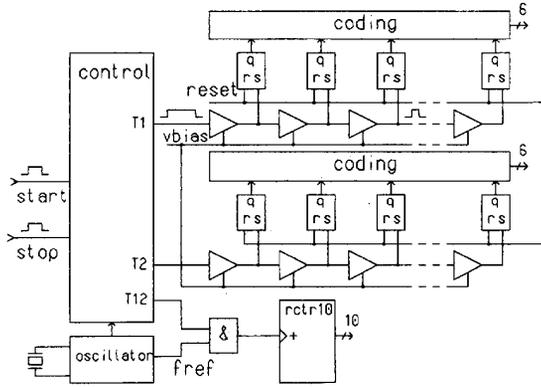
Fig. 4. Block diagram of the TDC.
