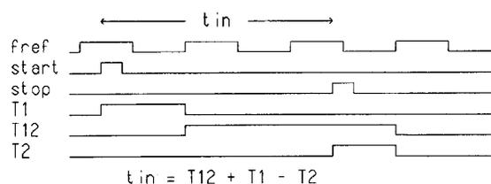
Fig. 2. Time interval measurement method based on the use of two separate interpolators.
