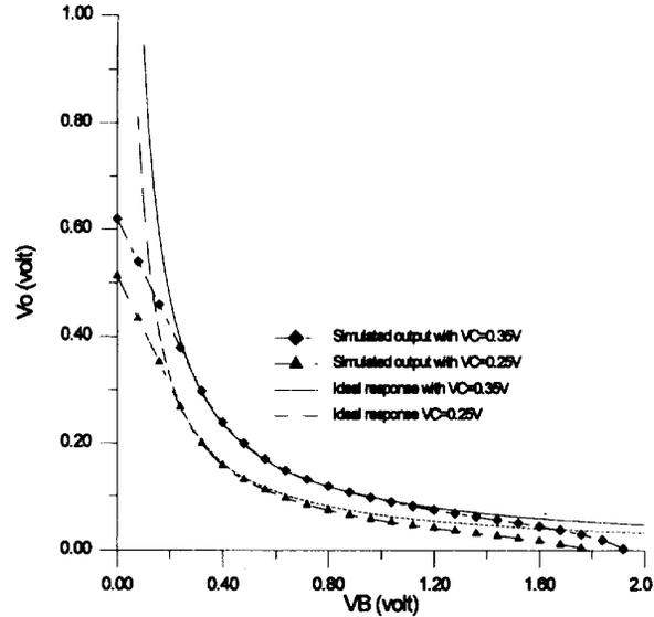
Fig. 4. The simulated transfer curves of Fig. 2 with  $V_C = 0.35 \text{ V}$  and  $0.25 \text{ V}$ .
