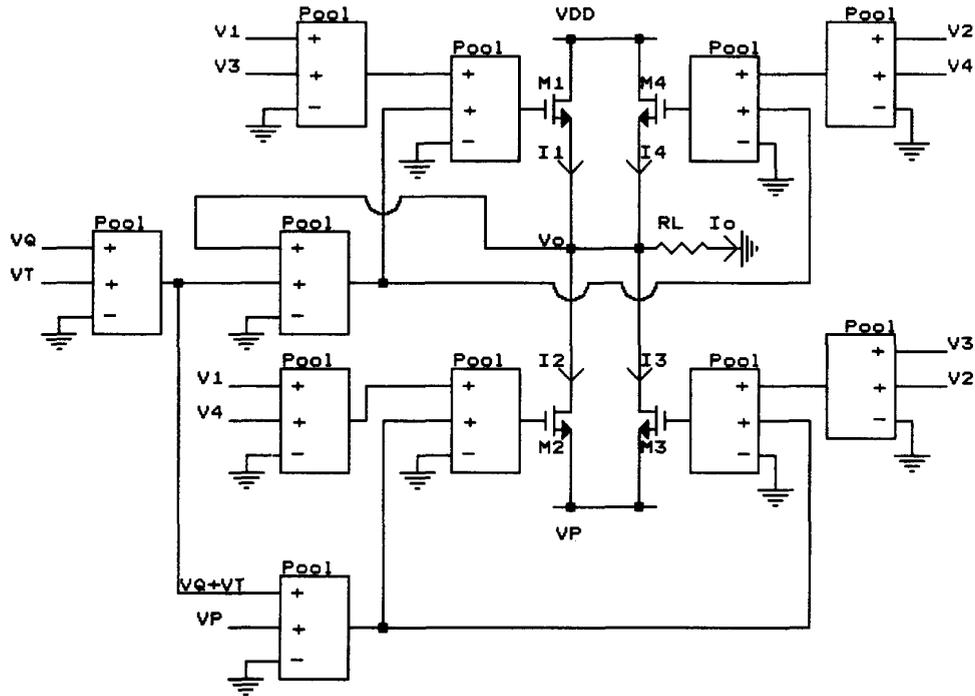
Fig. 3. The proposed four-quadrant multiplier.
