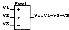
Fig. 1. The pool circuit proposed by Tsay and Newcomb.
