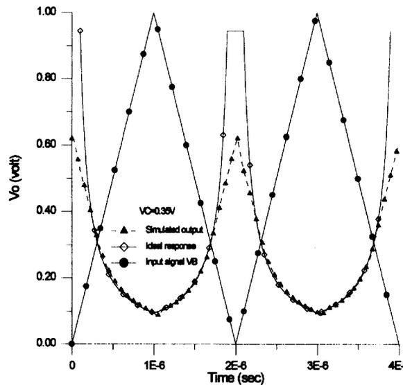
Fig. 5. A typical output waveform of Fig. 2 where a 0.5 MHz triangular signal changing from 0-1 V is applied to  $V_B$  and  $V_C = 0.35 \text{ V}$ .
