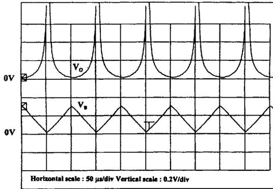
Fig. 7. A typical output waveform of Fig. 2 where  $V_B$  is a  $0.28 V_{p-p}$  triangular signal of 10 kHz with 0.14 V dc offset voltage. The horizontal scale is  $50 \mu\text{s}/\text{div}$  and the vertical scale is  $0.2 \text{ V}/\text{div}$ .
