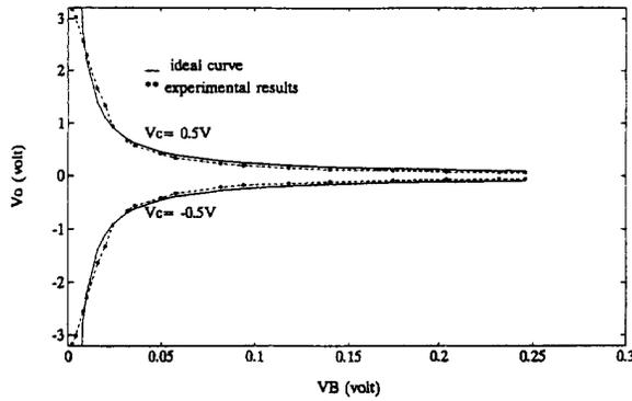
Fig. 6. The dc transfer functions of Fig. 2 with  $V_C = 0.5$  V and  $-0.5$  V.
