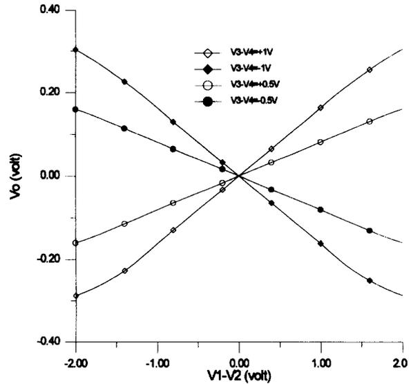
Fig. 8. The dc transfer curves of the proposed multiplier in Fig. 3 with  $V_1 = -V_2$ ,  $V_3 = -V_4$ ,  $V_Q = 1$  V,  $V_T = 1$  V, and  $R_L = 20 \text{ K}\Omega$ .  $V_3 - V_4$  changes from  $-1$  to  $1$  V and  $V_1 - V_2$  changes from  $2$  to  $-2$  V.
