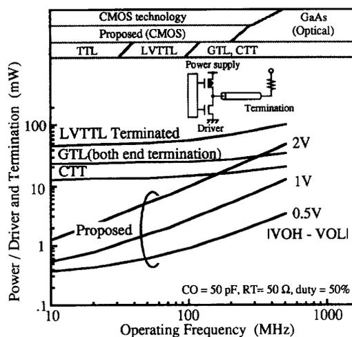
Fig. 1. Power comparison of interface circuits with termination.
