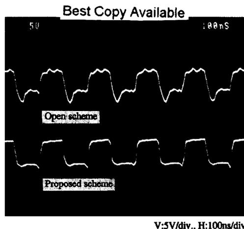
Fig. 6. Measured waveforms of the BiCMOS scheme.
