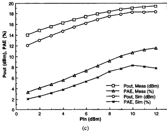
Fig. 7. The measured small signal gain and return losses as functions of frequency for (a) 21 sites of the single-stage push-pull PA, (b) 19 sites of the two-stage push-pull PA, and (c) the measured and simulated output power and PAE versus input power at 90 GHz for the two-stage push-pull PA.
