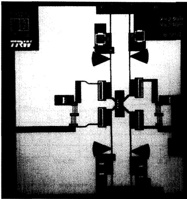
Fig. 3. The (a) schematic diagram. (b) Chip photograph for the single-stage W-band push-pull PA. The chip size is  $2.3 \times 2.4 \text{ mm}^2$ .
