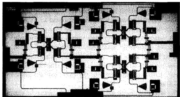
Fig. 4. (a) The block diagram of the two-stage push-pull PA. The schematic diagrams of (b) the first stage and (c) the second stage of the two-stage push-pull PA. (d) The chip photograph of the two-stage push-pull PA with chip size of  $4.4 \times 2.4 \text{ mm}^2$ .
