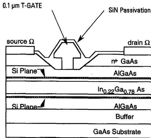
Fig. 1. Device cross section of the 0.1- $\mu\text{m}$  gate planar doped channel PM AlGaAs/InGaAs/GaAs power HEMT.
