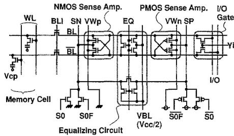
Fig. 1. Conventional sense circuit. This is the case that p-well under sense amp. is biased to GND.
