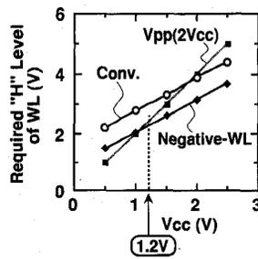
Fig. 10. Required WL's "H" level on negative-voltage WL and conventional method.
