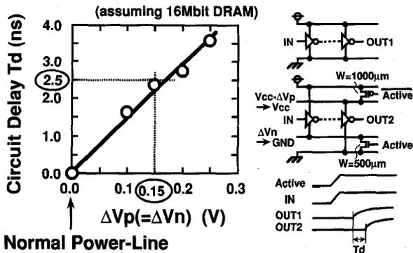
Fig. 5. Simulated circuit delay dependence on  $\Delta V_p (= \Delta V_n)$  assuming 16 Mb DRAM with hierarchical powerline structure. (30-stage inverters with  $L_n/W_n = 0.4 \mu\text{m}/10 \mu\text{m}$ ,  $L_p/W_p = 0.45 \mu\text{m}/20 \mu\text{m}$ ,  $FO = 5$  and local power line capacitance of 400 pF).
