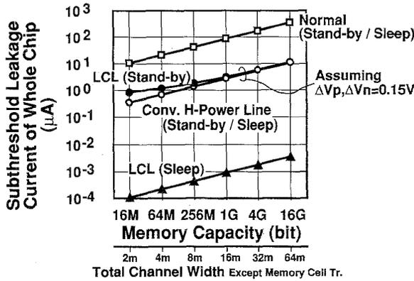
Fig. 7. Trend of subthreshold leakage current for normal power line, conventional hierarchical power line and LCL structure.
