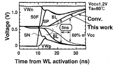
Fig. 3. Simulated waveforms of CTW sensing and conventional sensing. ( $V_{thn} = 0.4$  V @  $V_{bb} = -0.5$  V,  $V_{thp} = -0.5$  V, @  $V_{bb} = 0$  V).
