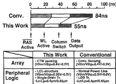
Fig. 8. Access time comparison between our work and conventional 16 Mb DRAM at 1.2 V and 80°C by simulation.
