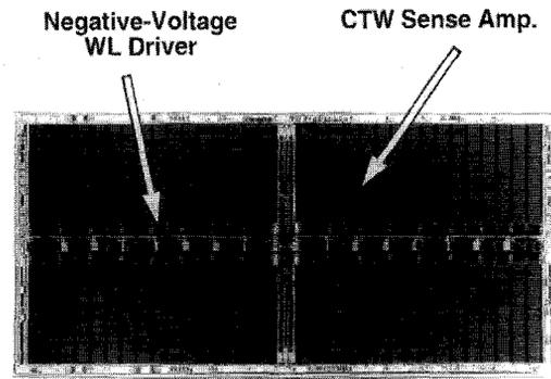
Fig. 12. Chip photo micrograph of experimental 16 Mb DRAM. Chip size is 7.9 mm  $\times$  16.7 mm.
