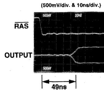
Fig. 13. Output waveform of experimental 16 Mb DRAM at  $V_{cc}$  to 1.2 V.
