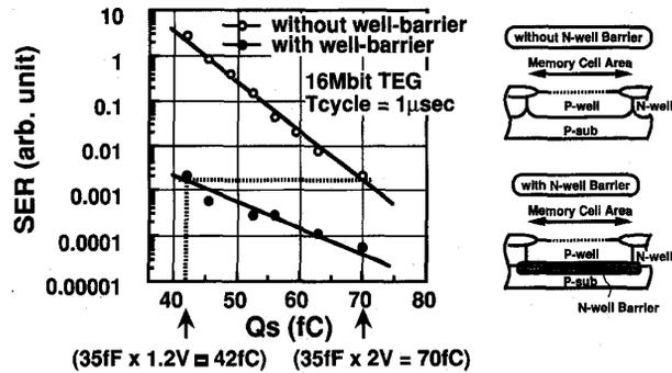
Fig. 11. Soft error comparison between with and without n-well barrier.
