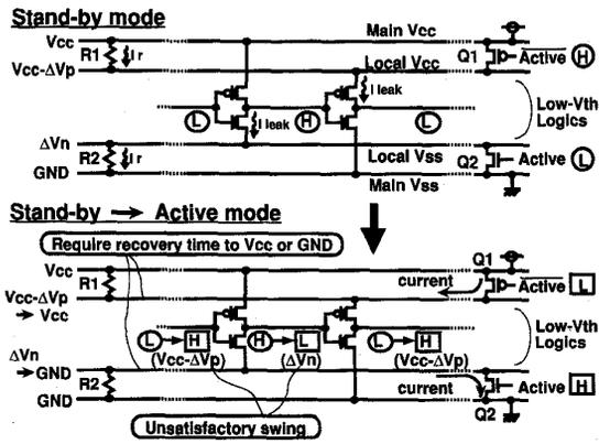
Fig. 4. Conventional hierarchical power line structure when entering active mode from stand-by mode.
