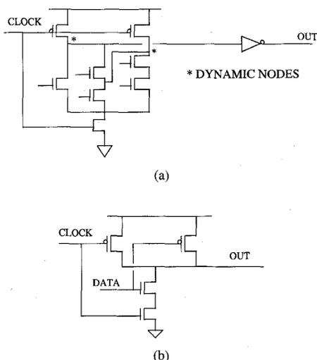
Fig. 1. (a) Domino-style dynamic gate. (b) Static clock-gating circuit.
