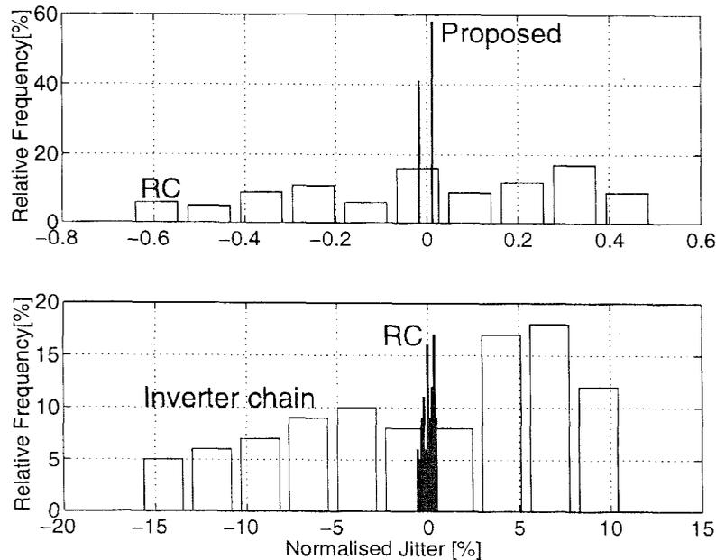
Fig. 12. Jitter histograms under power-line noise. Nominal  $t_d \approx 3.2$  ns at 2 V, 27°C.
