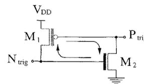
Fig. 1. Concept of the CMOS thyristor.
