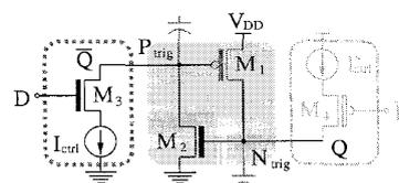
Fig. 2. Concept of the delay element based on the CMOS thyristor.
