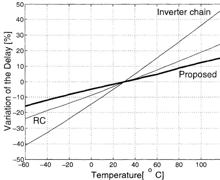
Fig. 11. Sensitivity to the temperature variation. Nominal  $t_d \approx 3.3$  ns at 3 V, 30°C.
