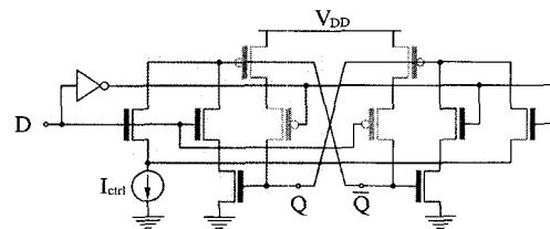
Fig. 6. Proposed delay element with static triggering.
