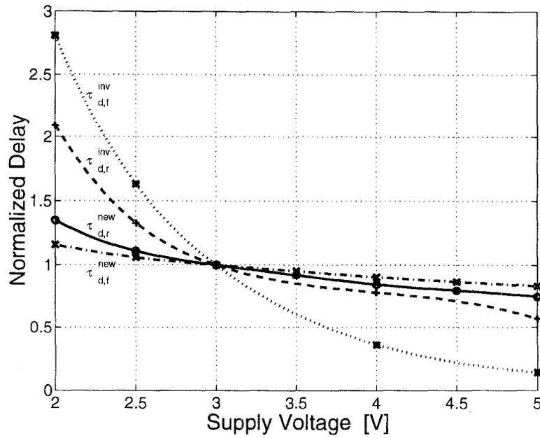
Fig. 10. Measured sensitivity to the supply voltage variation. The proposed delay element shows smaller sensitivity to  $V_{DD}$  in low voltage regime than inverter chain.
