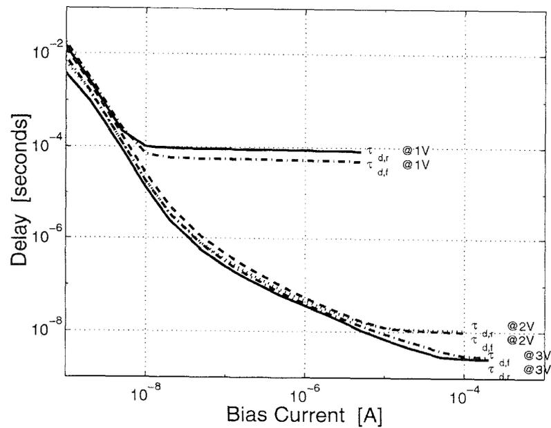
Fig. 8. Measured delay characteristics of the proposed delay element to  $I_{ctrl}$  and  $V_{DD}$ .
