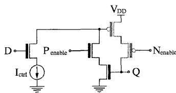
Fig. 4. Half-circuit of the delay element.
