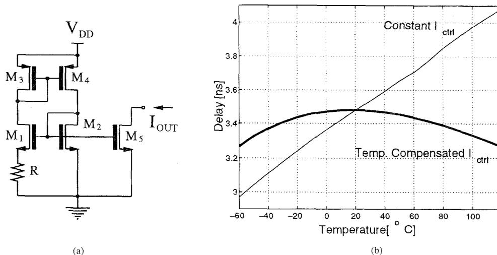
Fig. 13. Current source with a designed temperature coefficient. (a) Circuit Schematic. (b) Delay Response at  $V_{DD} = 3$  V.
