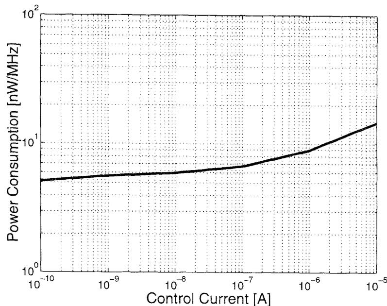
Fig. 9. Simulated power consumption of the proposed delay element to  $I_{ctrl}$ .
