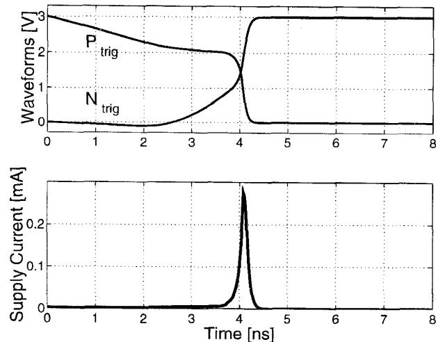
Fig. 3. Simulated waveforms and supply current of the delay element.
