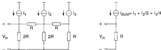
Fig. 4. Current-driven  $R$ - $2R$  ladder and Norton equivalent.
