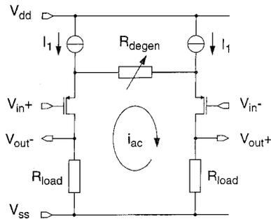
Fig. 2. Basic differential VGA architecture: degenerated differential pair with resistive loads.
