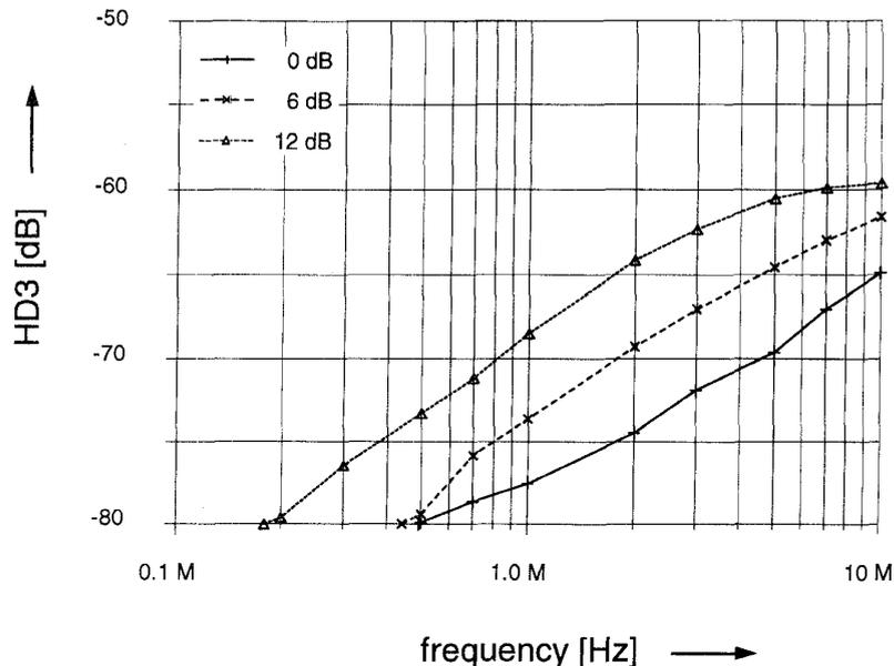
Fig. 10. Measured HD3 for single-sided inputs,  $1-V_{pp}$  output.
