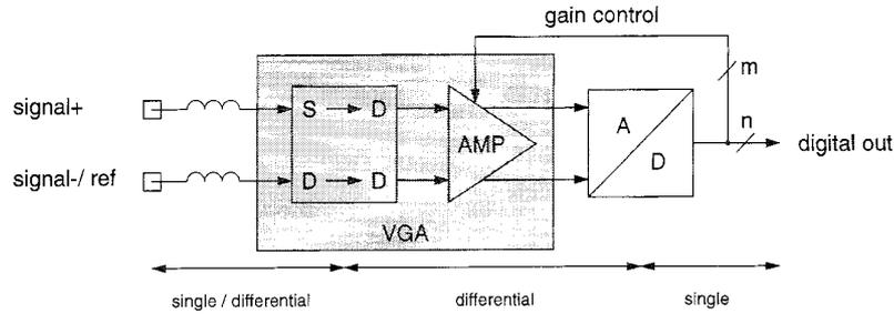
Fig. 1. Front-end for mixed-signal IC's.
