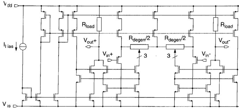
Fig. 6. Circuit implementation variable-gain amplifier.
