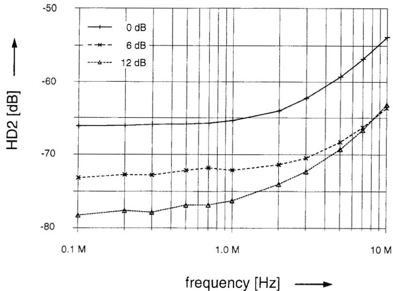
Fig. 9. Measured HD2 for single-sided inputs, 1- $V_{pp}$  output.
