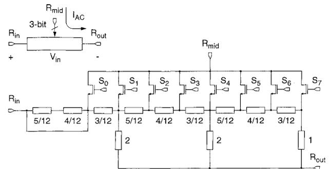
Fig. 5. Interpolated  $R$ - $2R$  ladder.
