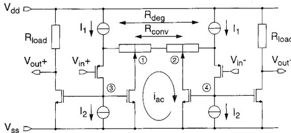
Fig. 3. Concept VGA with linear variable VI converter core.
