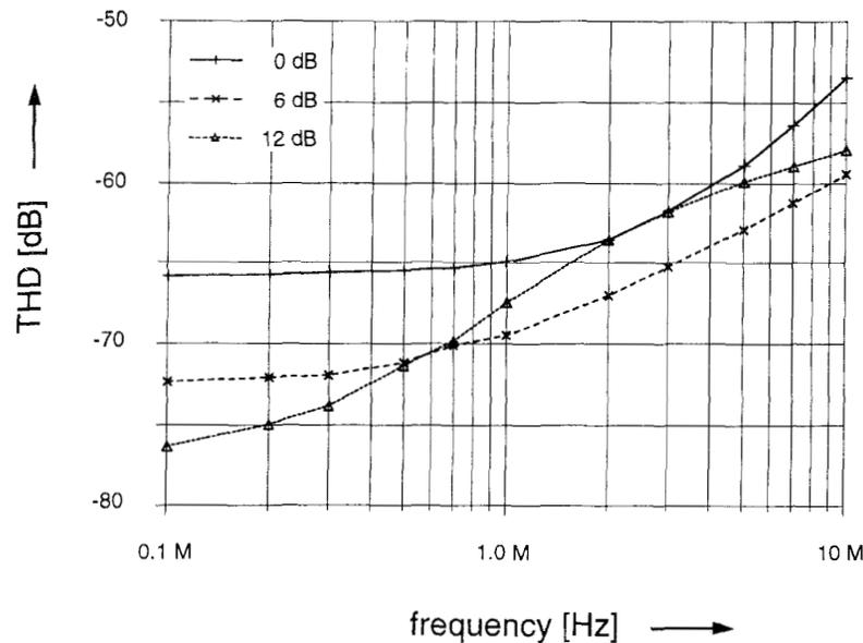
Fig. 11. Measured THD for single-sided inputs,  $1\text{-}V_{pp}$  output.
