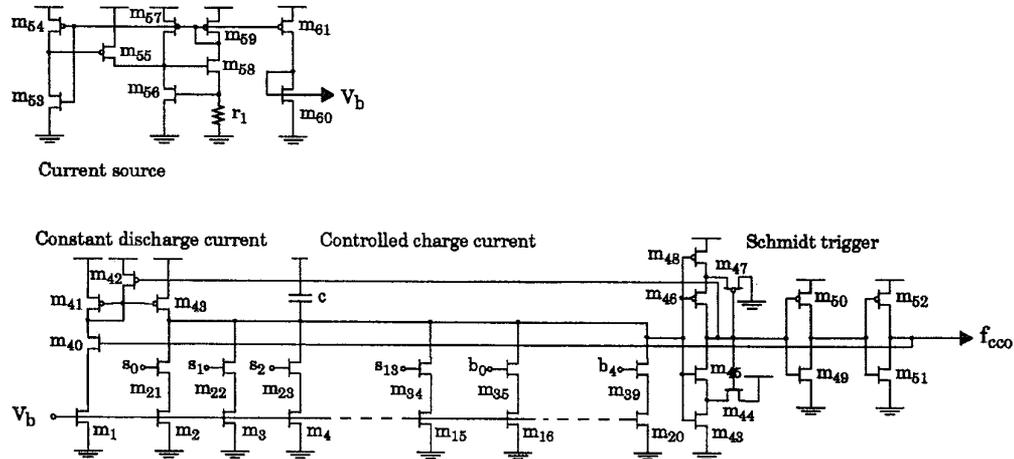
Fig. 2. Digitally controlled CCO.
