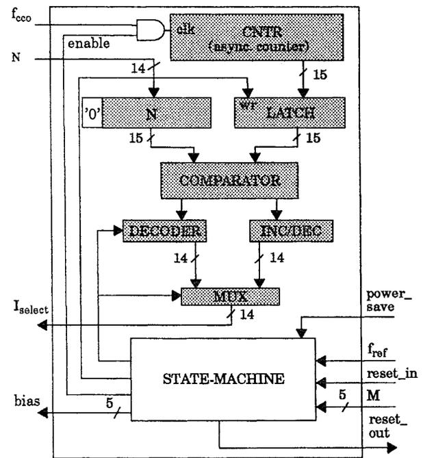
Fig. 3. Digital control of the CCO.
