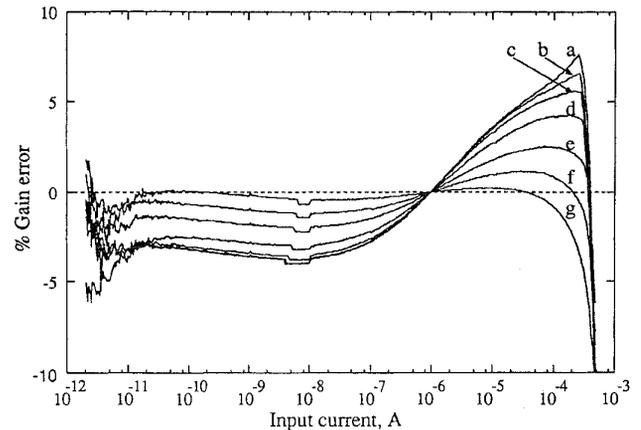
Fig. 10. Percent normalized gain error of the CMOS ACM using the ETP. Curves a-g correspond to  $(I_{CTRL1}, I_{CTRL2}) = (10^{-9} \text{ A}, 10^{-6} \text{ A}), (10^{-8} \text{ A}, 10^{-6} \text{ A}), (10^{-7} \text{ A}, 10^{-6} \text{ A}), (10^{-6} \text{ A}, 10^{-6} \text{ A}), (10^{-6} \text{ A}, 10^{-7} \text{ A}), (10^{-6} \text{ A}, 10^{-8} \text{ A}), (10^{-6} \text{ A}, 10^{-9} \text{ A})$ , respectively.
