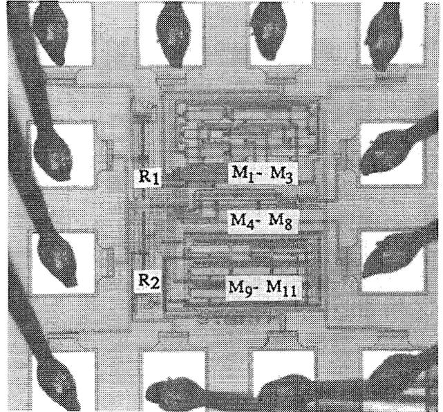
Fig. 5. Photomicrograph of the wide dynamic range CMOS ACM IC.
