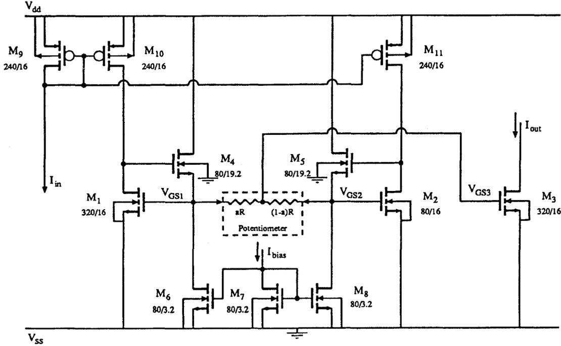
Fig. 1. CMOS adjustable current mirror.
