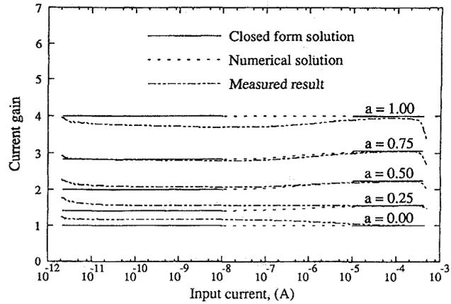
Fig. 7. Current gain of CMOS current mirror.
