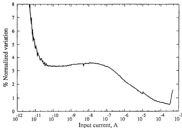
Fig. 8. Normalized gain variation among different IC's at  $a = 0.5$ .
