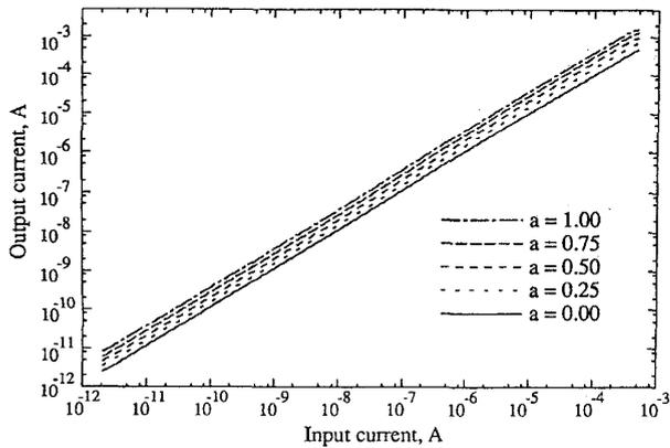
Fig. 6. Measured characteristics of CMOS current mirror.
