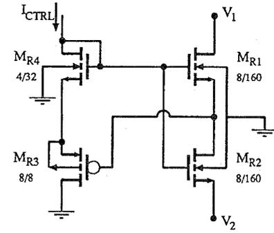
Fig. 4. Circuit diagram of the variable active resistor.
