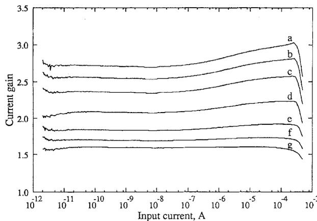
Fig. 9. Current gain of the CMOS current mirror using the integrated ETP. Curves a-g correspond to  $(I_{CTRL1}, I_{CTRL2}) = (10^{-9} \text{ A}, 10^{-6} \text{ A}), (10^{-8} \text{ A}, 10^{-6} \text{ A}), (10^{-7} \text{ A}, 10^{-6} \text{ A}), (10^{-6} \text{ A}, 10^{-6} \text{ A}), (10^{-6} \text{ A}, 10^{-7} \text{ A}), (10^{-6} \text{ A}, 10^{-8} \text{ A}), (10^{-6} \text{ A}, 10^{-9} \text{ A})$ , respectively.
