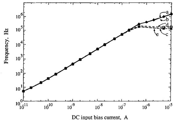
Fig. 13. Bandwidth of the CMOS ACM as a function of dc input current. Curve a corresponds to the gate of  $M_3$  shorted to the gate of  $M_2$ . Curve b corresponds to the gate of  $M_3$  shorted to the gate of  $M_1$ . Curves c, d, and e correspond to  $(I_{ctrl1}, I_{ctrl2}) = (10^{-8} \text{ A}, 10^{-6} \text{ A})$ ,  $(10^{-6} \text{ A}, 10^{-6} \text{ A})$ , and  $(10^{-6} \text{ A}, 10^{-8} \text{ A})$ , respectively.
