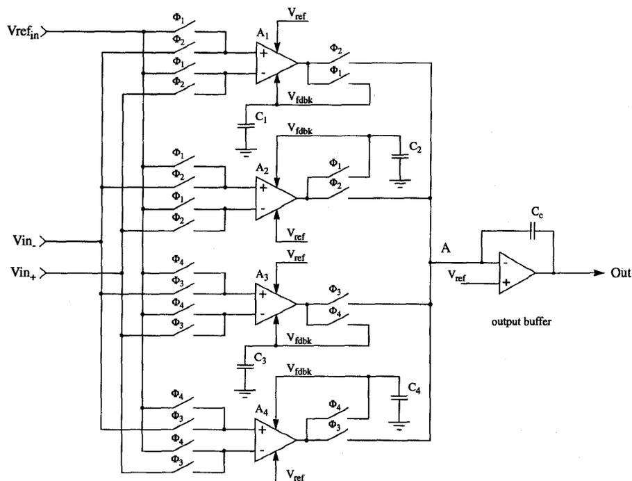
Fig. 1. Block diagram of the rail-to-rail ping-pong op-amp.
