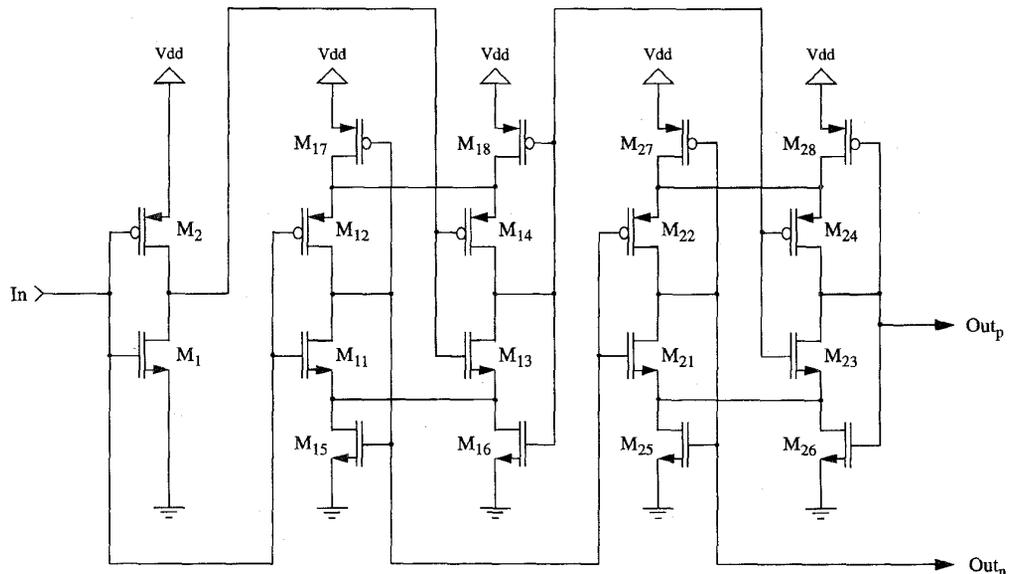
Fig. 4. Pseudodifferential CMOS switch driver.
