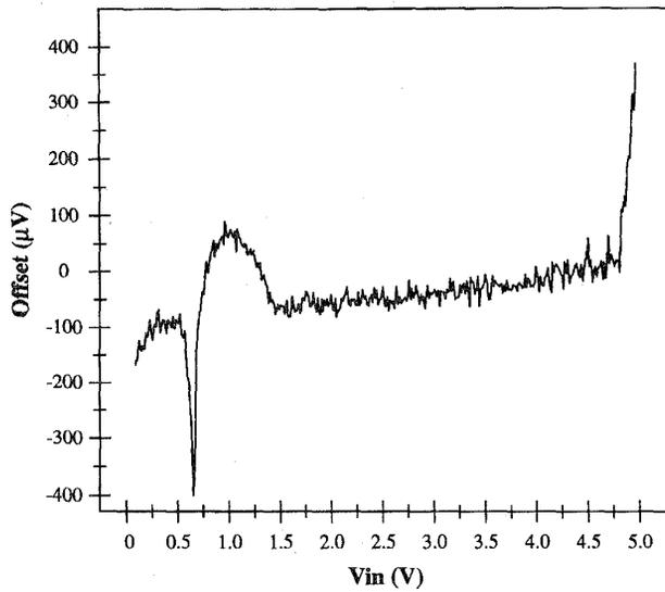
Fig. 9. Offset dependence on the input common mode voltage.
