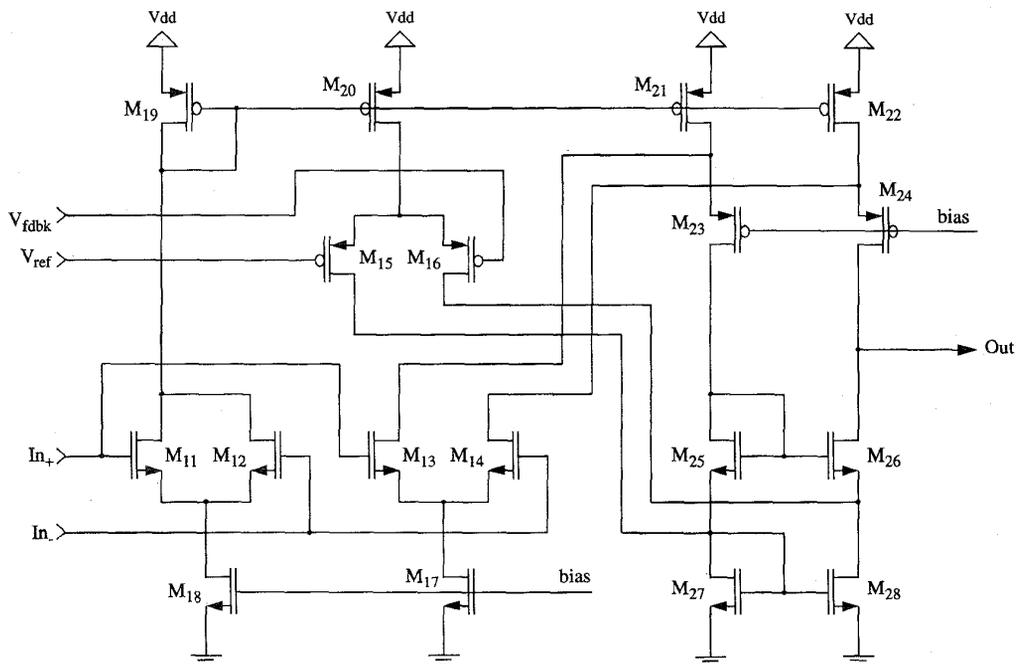
Fig. 3. Circuit schematic of the transconductance amplifier (nMOS inputs).
