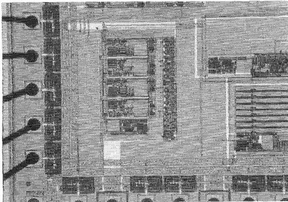
Fig. 6. Photomicrograph of the ping-pong op-amp.
