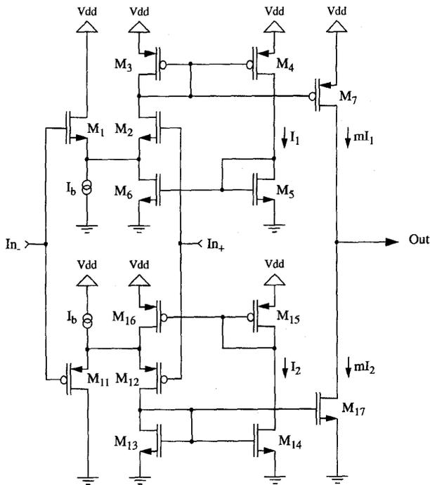
Fig. 5. Schematic diagram of the output buffer.
