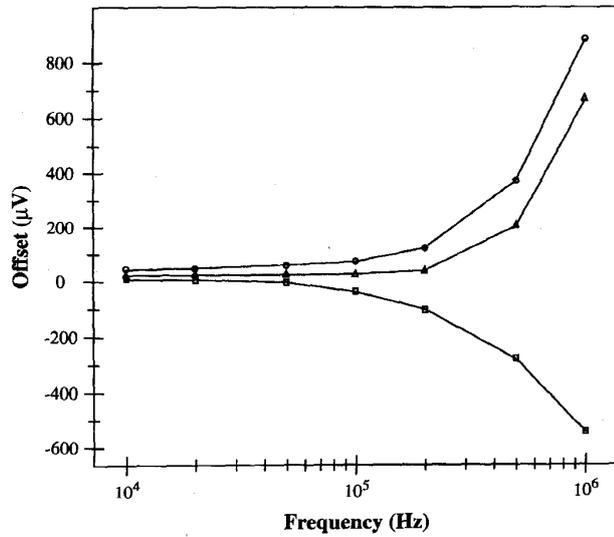
Fig. 7. Offset dependence on the clock frequency.
