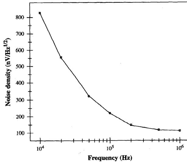
Fig. 8. Input referred noise floor versus clock frequency.
